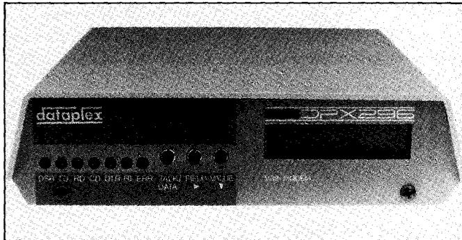
THE DPX-296 full duplex modem from Dataplex combines both the CCITT V.32 and V.22bis specification in a single unit, allowing communication at 9600 and 4800 bps while retaining full compatibility with 300, 1200 and 2400 bps.
