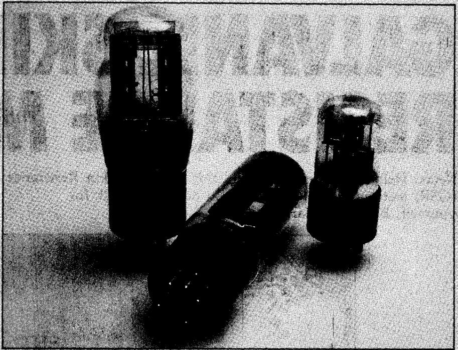
Some famous double diode valves. At left is the ubiquitous 80. Lying down is a much later version, the 5A5 – once widely used in TV receivers. At right is a 6X5 dual diode, a directly heated type with a common cathode used in detector applications. (All photos by John Lapke, valves courtesy of the Vintage Wireless Radio Company).
