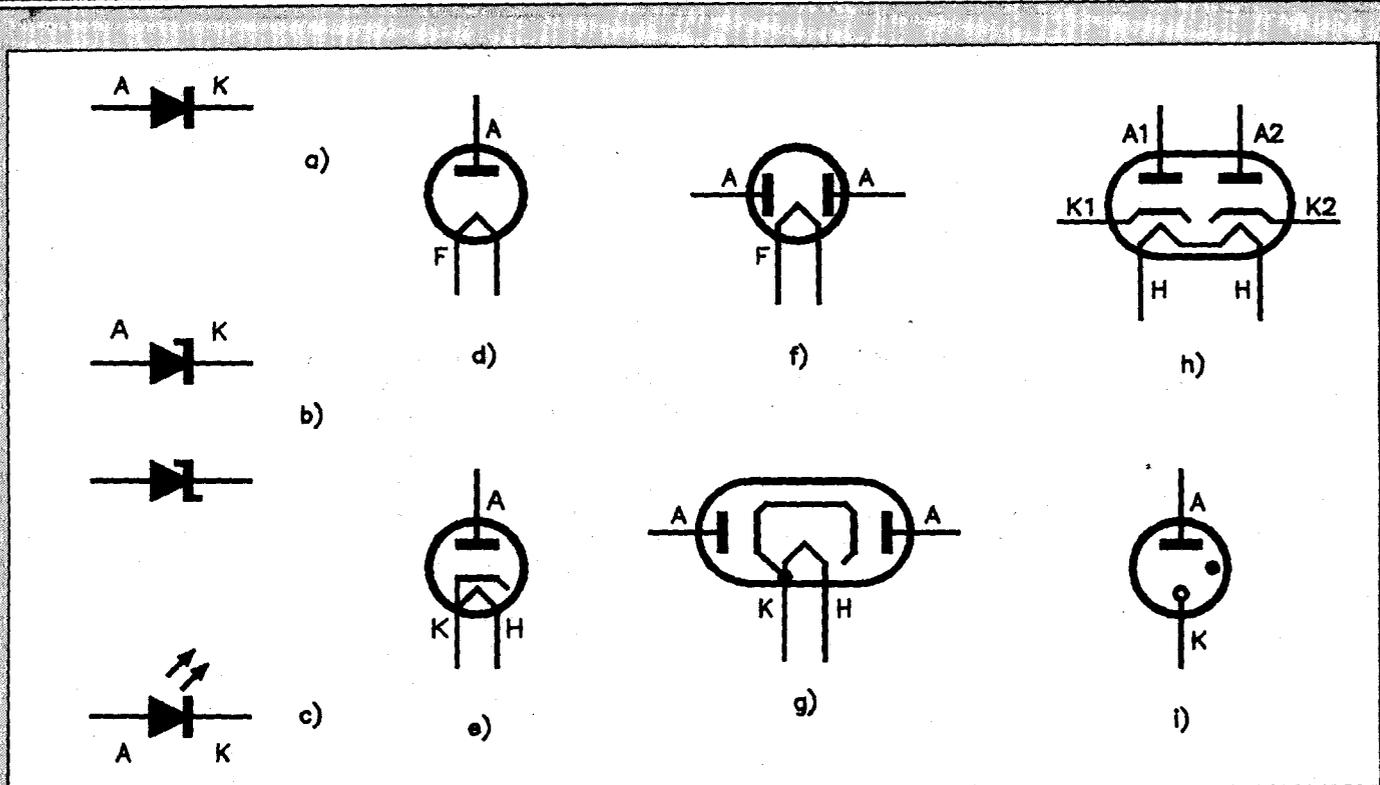
Figure 3.2 a) semiconductor diode; b) two symbols for a zener diode; c) light emitting diode; d) directly heated vacuum tube diode; e) indirectly heated vacuum tube diode; f) directly heated twin diode; g) indirectly heated twin diode; h) indirectly heated twin diode with separate cathodes. A = anode, C = cathode (some circuit diagrams use K for cathode), F = filament, H = heater.
