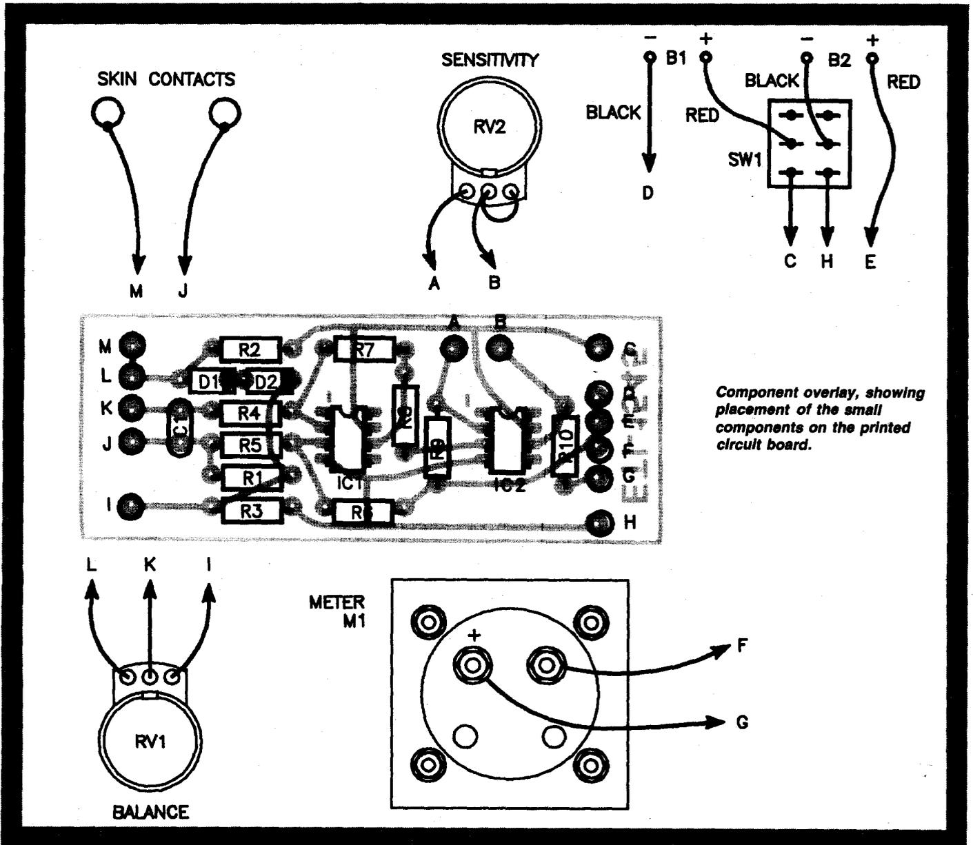
Component overlay, showing placement of the small components on the printed circuit board.
