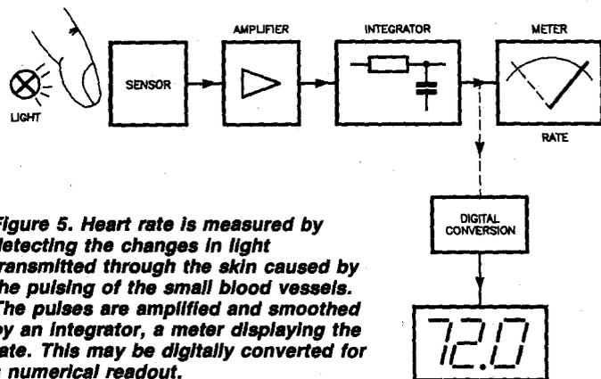
**Figure 5. Heart rate is measured by detecting the changes in light transmitted through the skin caused by the pulsing of the small blood vessels. The pulses are amplified and smoothed by an integrator, a meter displaying the rate. This may be digitally converted for a numerical readout.**
