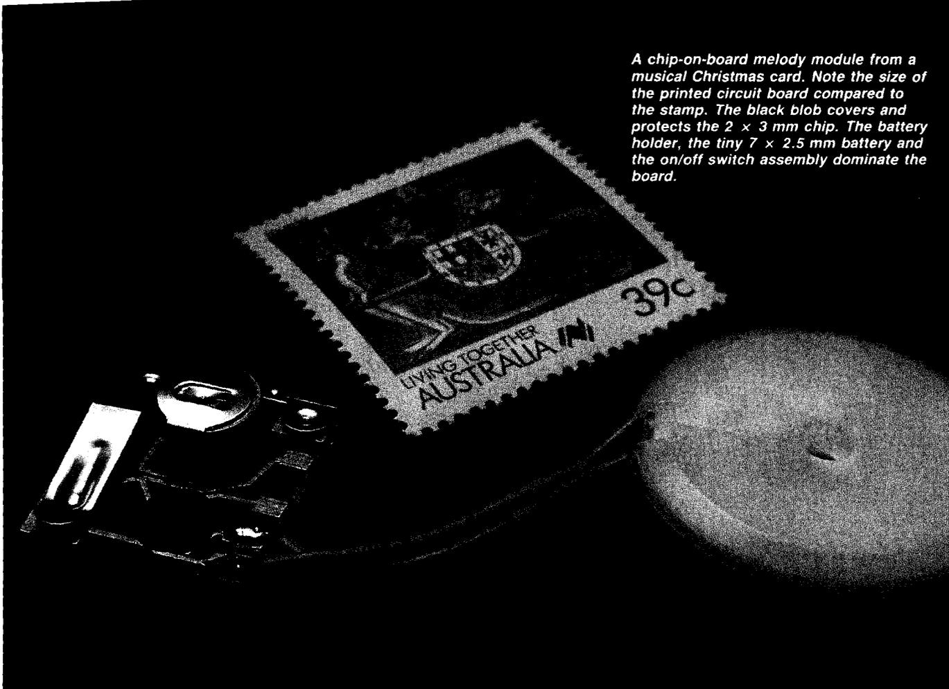
*A chip-on-board melody module from a musical Christmas card. Note the size of the printed circuit board compared to the stamp. The black blob covers and protects the 2 x 3 mm chip. The battery holder, the tiny 7 x 2.5 mm battery and the on/off switch assembly dominate the board.*
