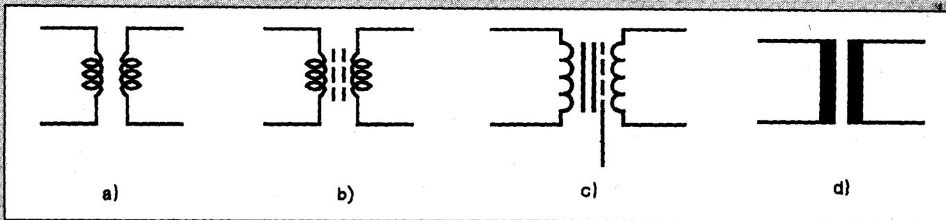
**Figure 3.1 Symbols for transformers.** a) untuned RF or IF transformer; a tuned version would have a capacitor connected across the secondary and/or primary; b) ferrite-cored transformer, RF, IF, or sometimes audio; c) iron-cored transformer, audio or power frequencies. The dashed line represents an electrostatic shield; d) power transformer.
