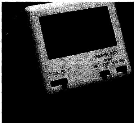
**Thought Technology's digital readout skin temperature meter. It also provides an audio tone output and boasts resolution of 0.1 degree on the readout, 0.05 degrees audible.**
