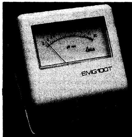
**The Thought Technology electromyogram features two ranges and audible tone feedback.**
