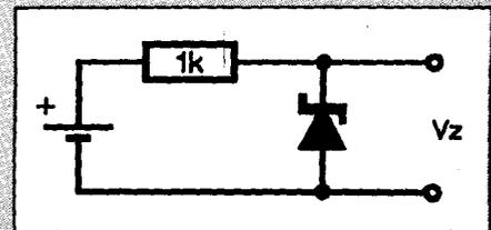
Figure 3.3. Simple circuit for testing zener diodes. The battery (or power supply) voltage should be 6 V greater than the expected zener voltage.
