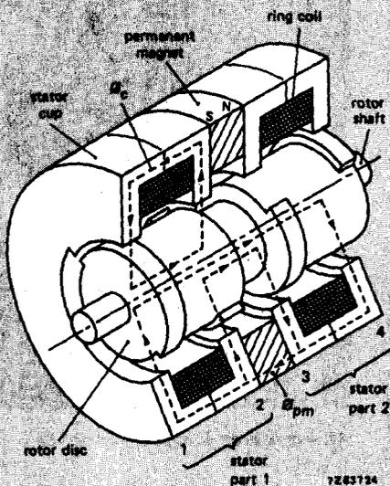
Figure 5a. Ring coil hybrid stepping motor, showing the paths of the permanent-magnet flux  $\phi_{pm}$  and coil flux  $\phi_c$  for one coil excitation mode. For this mode  $\phi_c$  adds to  $\phi_{pm}$  in disc 1 and subtracts from it in disc 2.
