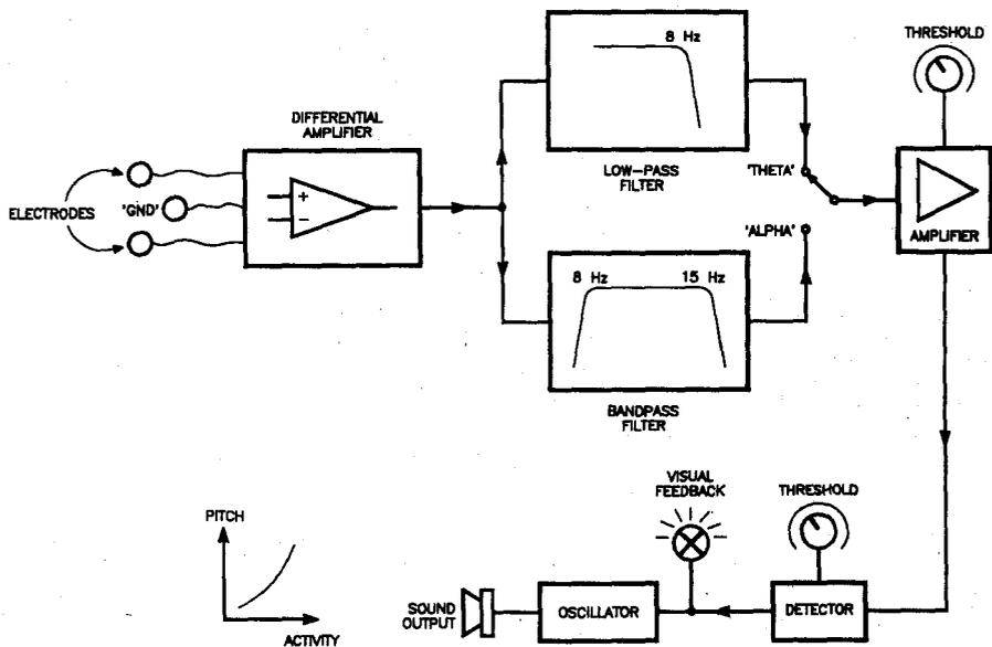
of low amplitude, measuring a few microvolts, the signals can be quite easily sensed using electrodes on the skin and filters to select the desired brain wave pattern. Figure 6 shows a typical brain wave biofeedback instrument.
