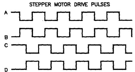
Figure 2. Showing the operating pulses required by unipolar stepping motors. The A-B-C-D pulse sequence is output from pins 6, 8, 9 and 11, respectively, of the SAA1027 in the controller circuit.
