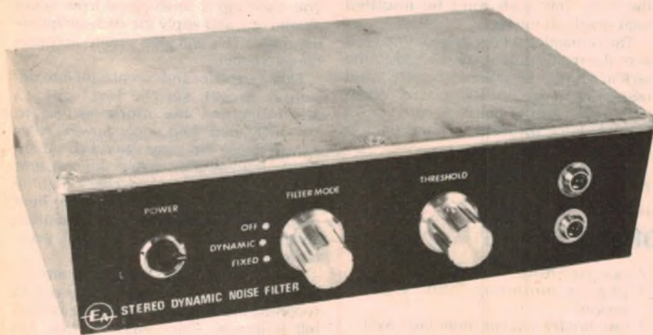
High level signals switch the filter circuits out and extinguish the two LED indicators.
