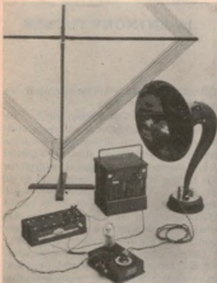
Fig. 3: the Loewe OE333 IC radio with batteries, frame aerial and speaker.
