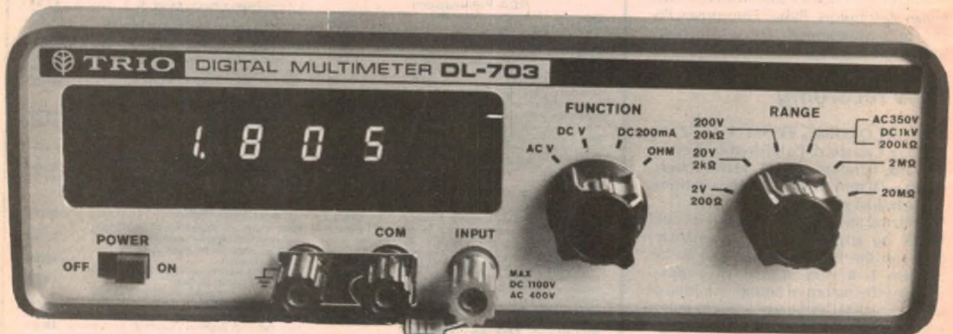
This photo shows the panel almost full size. It is shown here measuring a 1.8k resistor.
