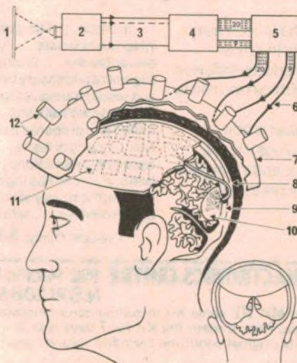
Principle of the proposed 180-point visual prosthesis system: 1—pattern; 2—picture source; 3—180 video signal lines; 4—implant driver logic; 5—modulators; 6—pulse amplitude modulation signal; 7—removable transmitter hat; 8—scalp; 9—skull; 10—rubber cap with electrodes; 11—implant with receivers and AND gates; 12—inductive loop transmitters.
