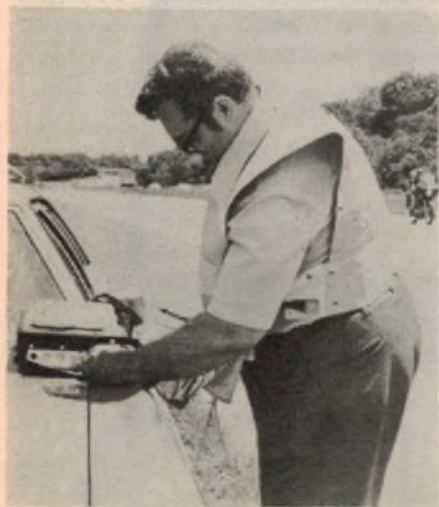
Kenney attaching the transducer cable to the tape recorder used to record the noise vibrations of oncoming traffic.
