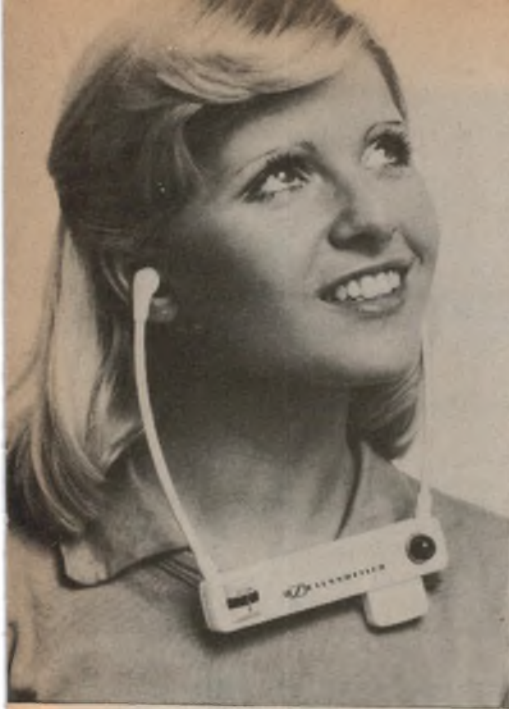
The Sennheiser HDI 406 headset which receives its signal via modulated infra-red light entering through the filter bezel on the right. The switch/volume control is on the left while the tiny unit underneath is the plug-in battery pack and charger.
