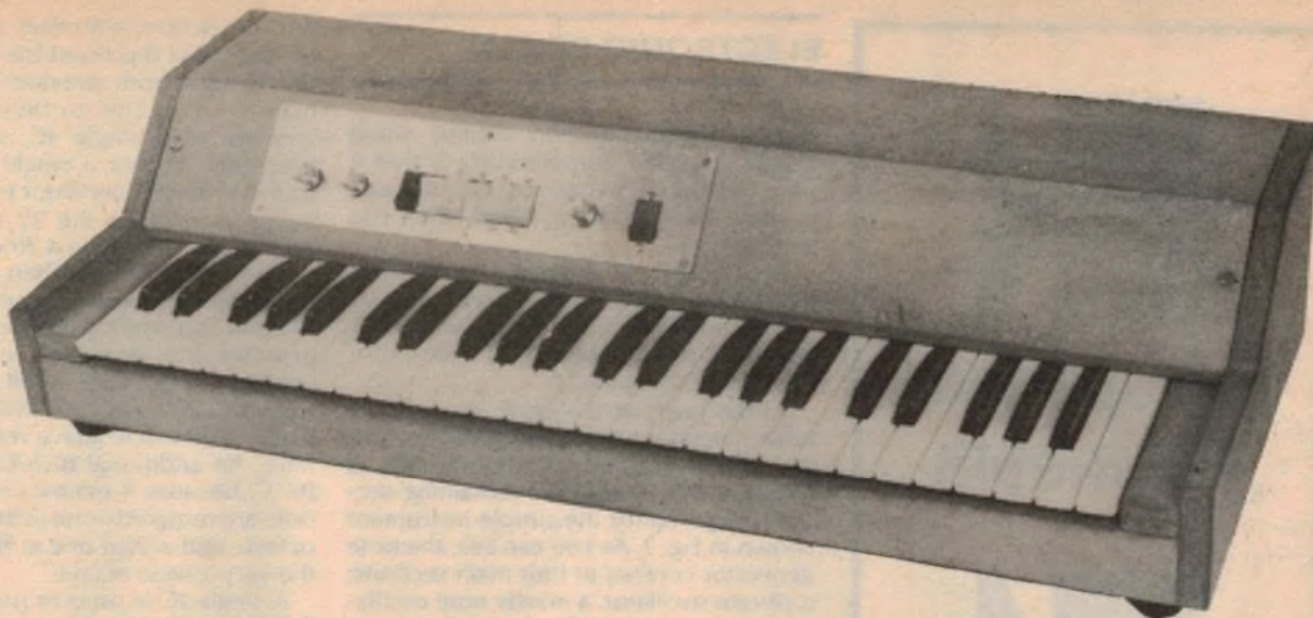
Above is the simple organ, photographed before it was completed by the addition of a lettered front panel and music rack. Below is a view of the note generator board, which actually provides all 97 notes required for quite pretentious organs.
