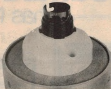
Above: The batten lamp holder, mounted on the loose-fitting top "plug", which in turn is held in place by three countersunk head woodscrews. Below: The component layout, shown on the PCB pattern, which is reproduced actual size to facilitate tracing.
