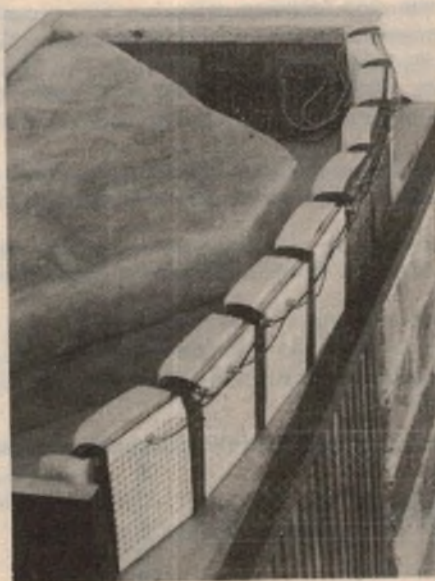
Fig. 12. Electrostatic speaker cavity, with cover removed, fitted to the top of the brick bass vented enclosure.
