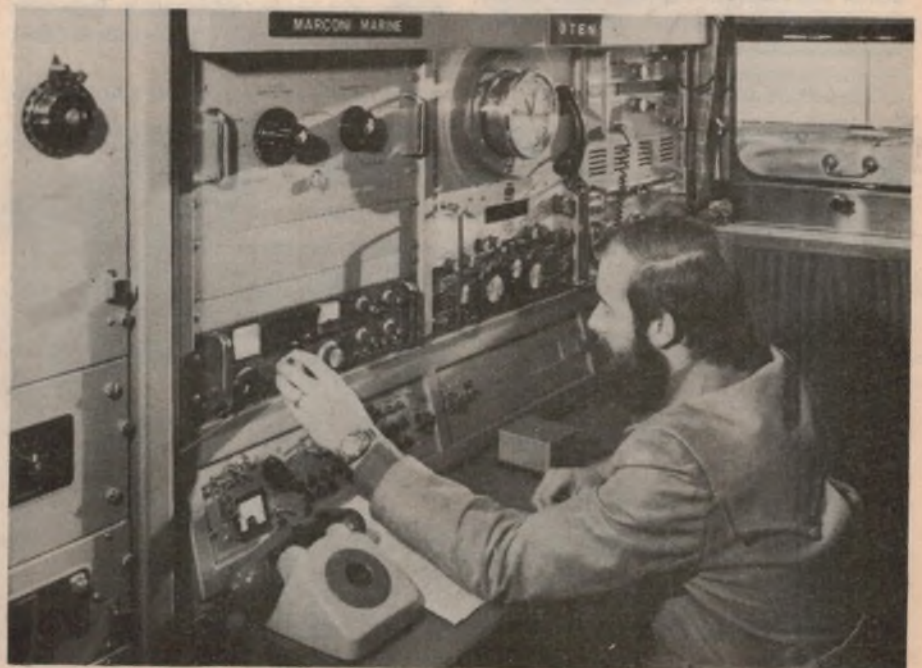
The radio room of a modern trawler. The Polish-built Boyd Line "Arctic Buccaneer" has a complete Marconi Marine communications station.
