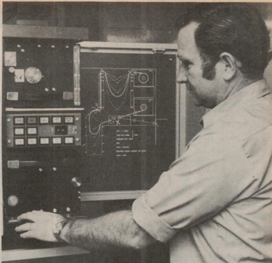
The output end of the Digiset currently in use at Broadway. The two later models will each be capable of producing a full broadsheet page every 90 seconds.
