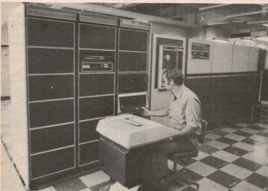
The Digiset photo-typesetter is capable of setting 40 lines of type a second.
