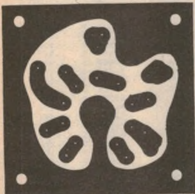
Fig. 7: actual size artwork for the PC board.
