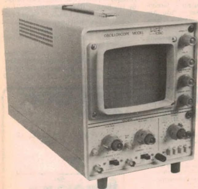
*Good control layout is a feature of the BWD 539C. It has bandwidth of 20MHz and maximum sensitivity of 10mV/cm.*
