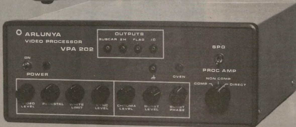
The Arlunya video processing system comprising the SPG.200 Sync Pulse Generator and the VPA.202 Video Processor will accept signals from any 625/50 PAL source, in particular from VTR's. It will clean up these signals by completely regenerating the blanking sync and burst components of the signal. System level, chroma level, white limit level, sync pulse amplitude, burst amplitude and phase can all be varied by front panel controls or remote DC voltages.
