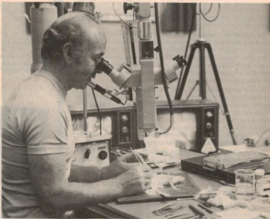
Dr Earl Owen, who conducted the International Microsurgery Workshop, is shown using the motorised operating microscope. The compact Hitachi colour TV camera is integrally fitted to the viewing optics.
