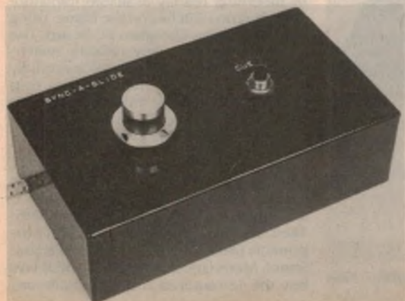
The prototype unit, built into a plastic utility case. The cue control button is on the right, while at left is the PLL frequency adjustment control.
