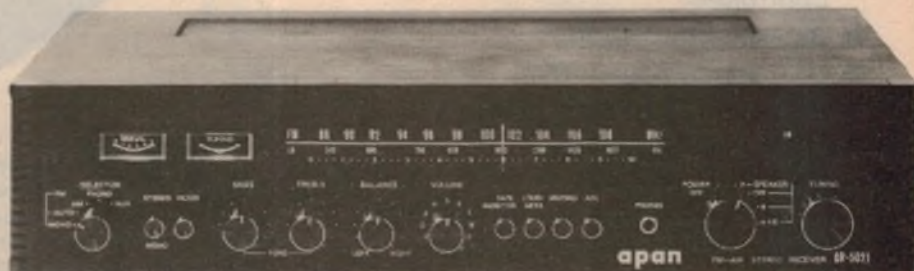
Claimed to be “eminently suitable for Australian conditions”, this new APAN AM/FM-stereo receiver, with AFC, offers 35W RMS per channel into 8 ohms, with both channels driven. It provides access for phono and tape, switching for two pairs of loudspeakers, twin tuning meters, well illuminated dial and generous control facilities. Specifications are good and the distributors claim that it represents outstanding value for their recommended retail price of $299. For further information and specifications: Mr P. Harris, Ralmar Agencies Pty Ltd, 71-73 Chandos St, St Leonards, NSW 2065.
