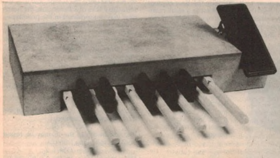
The prototype pedal unit, which includes a swell pedal. The article explains how to provide it with either a single stop or a number of stops.
