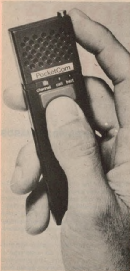
The PocketCom miniature CB transceiver, shown about two-thirds actual size. It offers beep tone paging and 100mW output.
