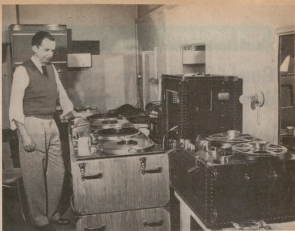
Mullin in 1950 with two "portable" Model 200 Ampex tape recorders and the first Model 300 to leave the factory. With these machines, Mullin had available a full range of advanced editing techniques.
