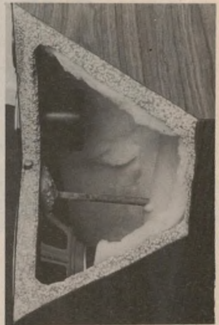
This cutaway section from one of the George Hawthorn enclosures clearly shows the polystyrene beads in the concrete mix from which the enclosure is cast. Note also the internal steel bracing rod and the lining on the inner surface. Synthetic woodgrain material on the outer surface gives a convincing timber finish, although plain black or white is also available on order.
