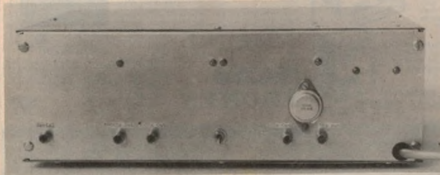
Rear view of the prototype. The five sockets (from left to right) are: aerial input, 100kHz out, 100Hz out, 50Hz out and 1Hz out. The switch is for battery on/off.
