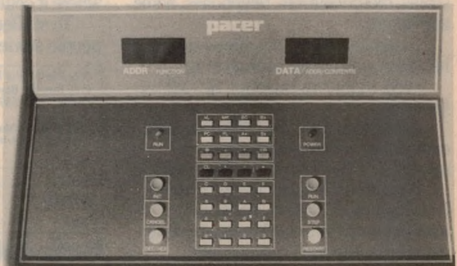
This is the PACER control panel. Hexadecimal numbers are entered via the lower 16 keys, while the upper 16 are used for control. The alphanumeric displays are at the top.
