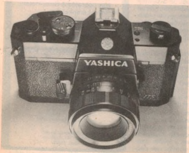
Through-the-lens metering is employed by the Yashica TL Electro X single lens reflex camera. An integrated circuit controls the shutter speed, which can be varied from 2 seconds to 1/1000 second.
