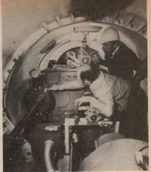
Inside the gear-packed fiberglass capsule atop the 100ft tower author Kocivar gets a close look at the hefty disc brake that keeps the giant rotor stationary when adjustments are being made.
