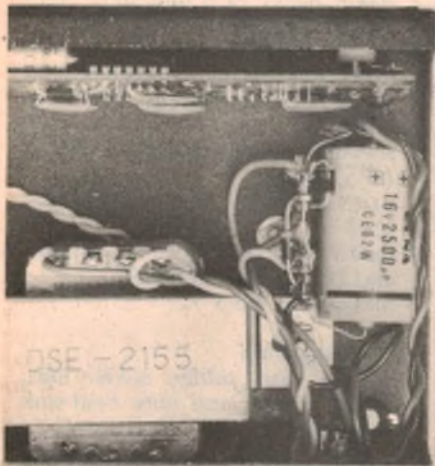
ABOVE: This photograph shows the layout of the power supply components. Note the regulator at the rear.
