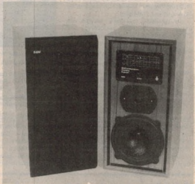
The black foam front of the DM5 peels off to reveal the two loudspeakers on the baffle. Below is one of the individual frequency response plots supplied with our sample pair of DM5's.
