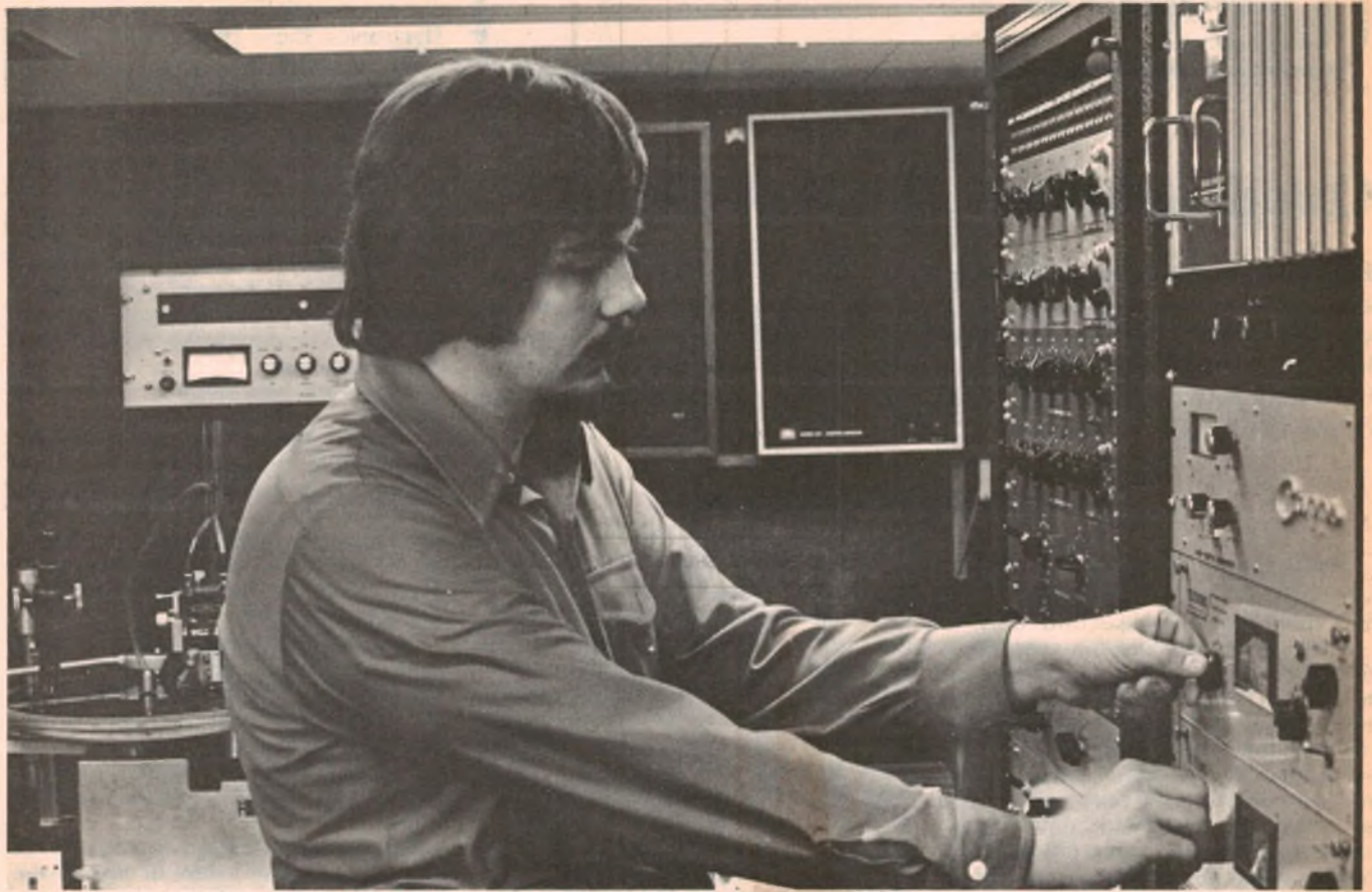
“Carl Rowatti, Chief Engineer, adjusting the Program limiters prior to cutting a master lacquer”.
