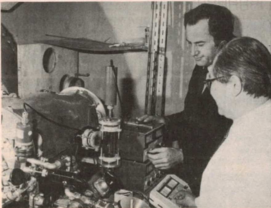
Professor D. J. Bradley (left) and a member of his research team demonstrate the new laser. Pulses as short as one third of a picosecond can be produced.
