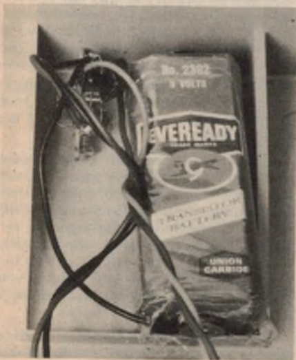
This view shows the simple power supply regulator mounted next to the battery. The necessary components are mounted on a piece of 5-tag strip.
