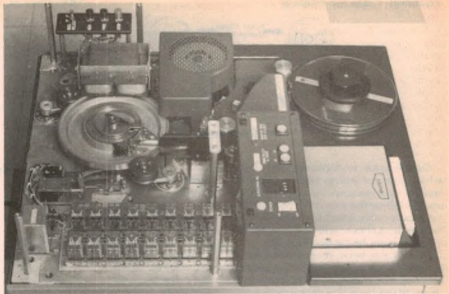
The open reel version copier with cover removed. The coaxial reel is clearly visible on the left with the AC field magnets directly above it. The master tape (cartridge) and the slave tape (reel) are on the right.
