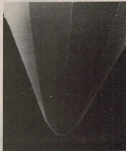
A microphotograph of a parabolic stylus also magnified 1850 times. Note the two shoulders, forming an angle of 90 degrees, which sit snugly against the walls of the groove,
