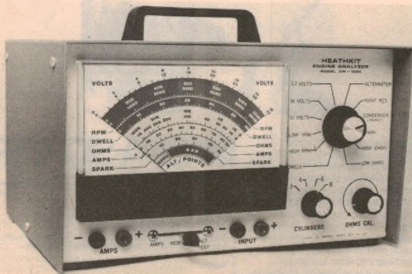
A comprehensive range of measuring facilities makes the CM-1050 Engine Analyser an invaluable service tool for engine tune-ups and fault finding.
