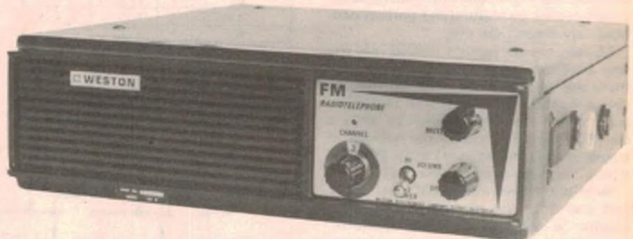
A typical mobile marine FM radio telephone unit as approved by the PMG's Department. It operates from a 12V DC supply, generates 25W RF output, and can provide up to 10 channels. (Photo courtesy Weston Electronics Pty Ltd.)
