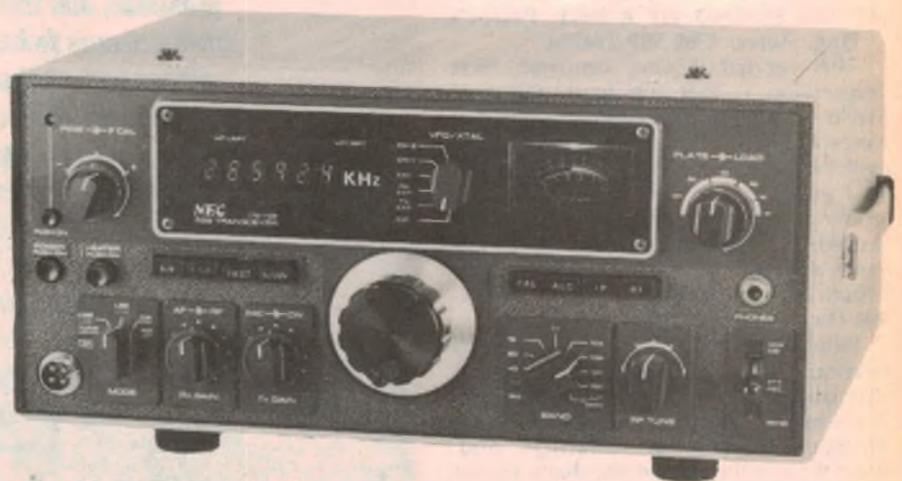
The digital frequency meter readout is to the left of the upper panel, with the VFO/XTAL switch and monitor meter to the right. The lower controls are, L to R, Mode, Rx Gain, Tx Gain, Band, RF Tune, and PTT/VOX, etc.
