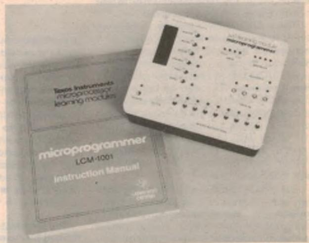
module is designed to demonstrate, using the SBP 0400 device as an example. Each of the control inputs, data inputs and data outputs of the device are brought out the LED indicators, and all inputs are provided with miniature toggle switches so that the device may be manually programmed. A pushbutton provides the clock signal input.
