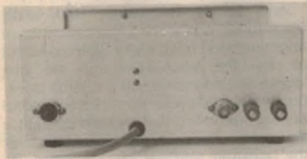
A view of the rear panel. The speaker socket is at left, with the aerial socket and terminals to the right.
