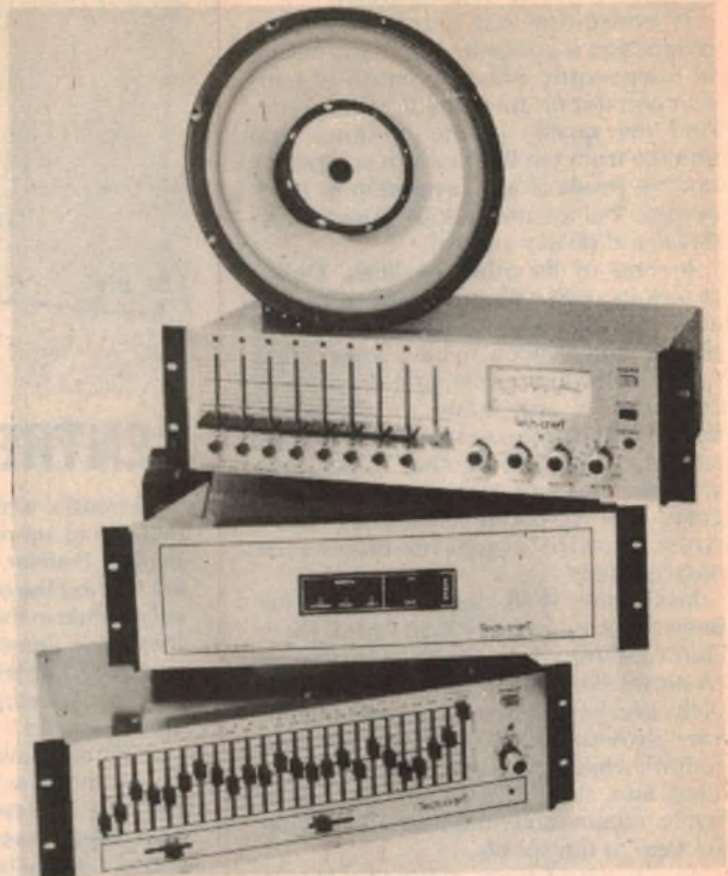
From the top: A Tech-craft dual concentric loudspeaker; the TCM 200 8-channel mixer; TCB 125 125W solid-state power amplifier; TCE 200 spectrum equaliser.
