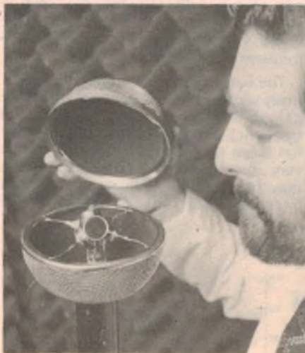
Is this the microphone hifi purists should really be backing—the tetrahedral design which is the basis for the British "Ambisonic" multi-channel system? (IMF Products, C.B., Westbourne St, High Wycombe, Bucks, England.)
