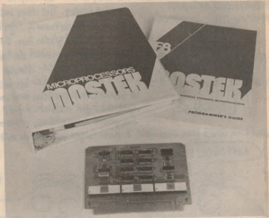
This is the Mostek F8 evaluation kit, comprising PCB, a binder with user manuals, and a programmer's guide. The CPU clock is crystal controlled.
