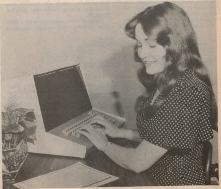
Apart from the power supply, the Sphere 320 is fully self-contained.
