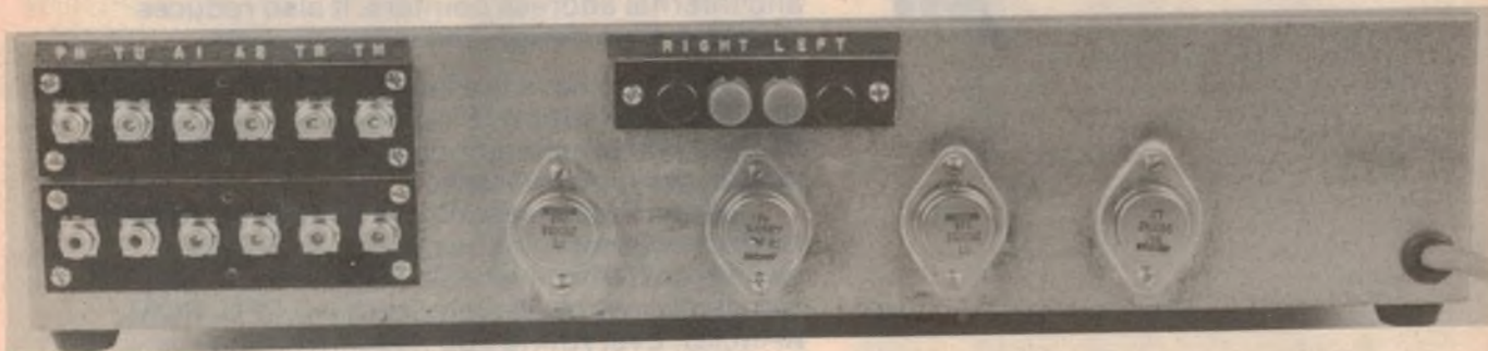
Note how the thermal compensation transistors are positioned on the rear panel. Below is the rear of the chassis.
