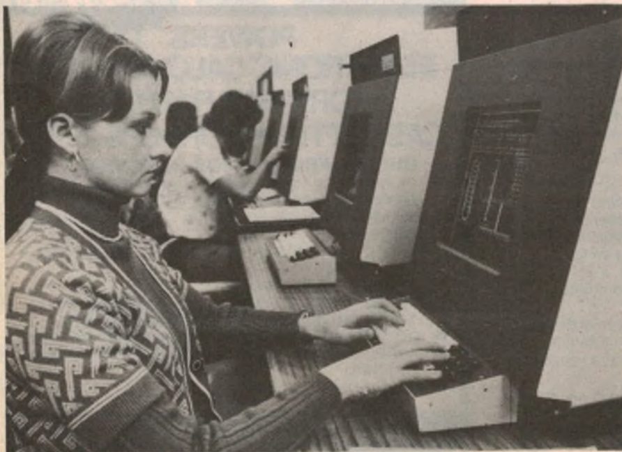
Students using the CDC PLATO computer-based education system. The system distributes instructional materials in the form of text, numbers, animated drawings and other graphics for individualised, self-paced learning.
