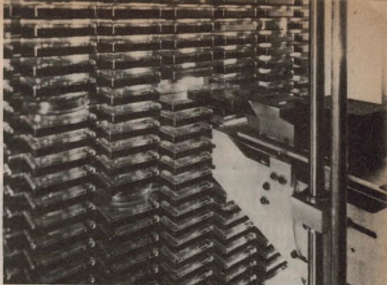
A close-up view of the CUERAC 500-slot cartridge library and the servo controlled "gripper" mechanism which transports selected cartridges to and from the playing decks. Adjustments permit cartridges to be positioned accurately within each slot.
