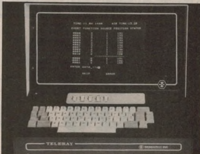
The visual display terminal, with its ASCII keyboard and, on the screen, the display of a typical program format. While just figures to the casual observer, the readout gives a detailed rundown on events (and non-events!) to an operator accustomed to the coding.
