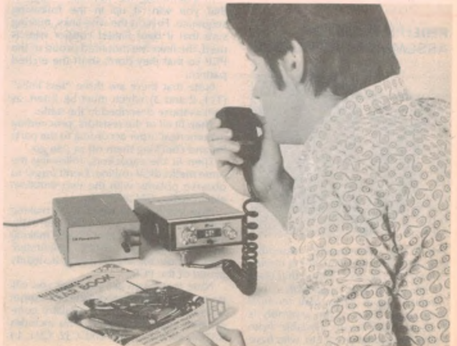
Powermate will run most CB transceivers with a maximum output rating of 5W.
