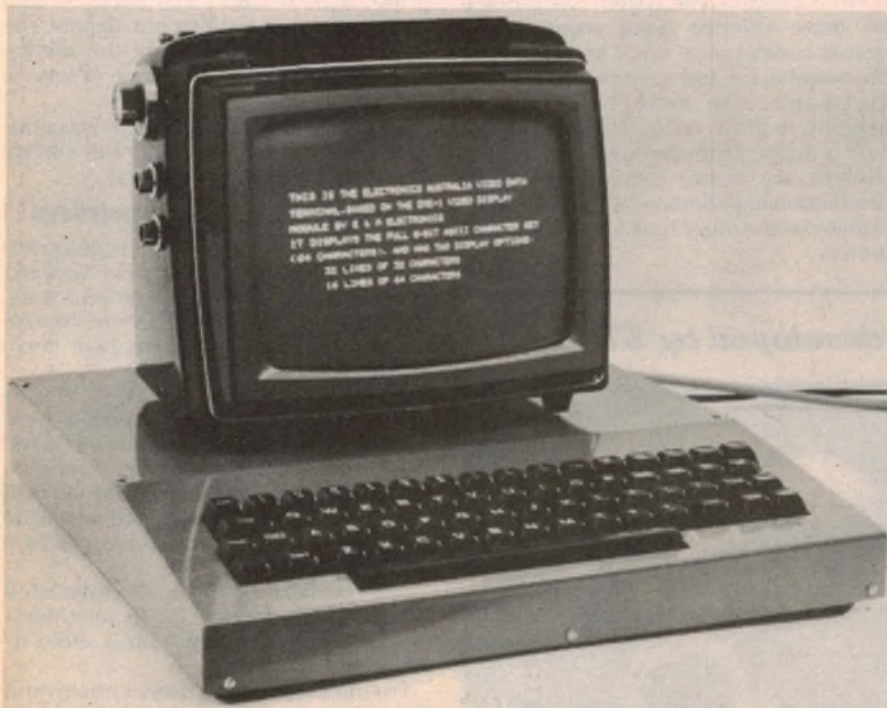
Here is the complete terminal, with a 21-cm portable TV receiver used as the display device. The low-profile case was kindly provided by Cowper Sheetmetal & Engineering, of 11 Cowper St, Granville, NSW.
