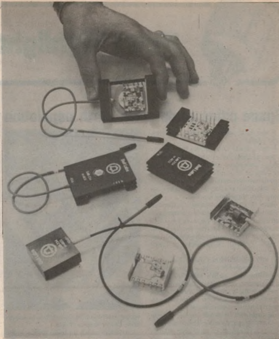
Shown are laser transmitter and receiver packages manufactured by Bell Labs for lightwave communications. The two packages making up the transmitter are at top. The package being held contains a laser, a chip no larger than a grain of salt, which is used to create the tiny pulses of light that carry information through the hair-thin optical glass fibres.
