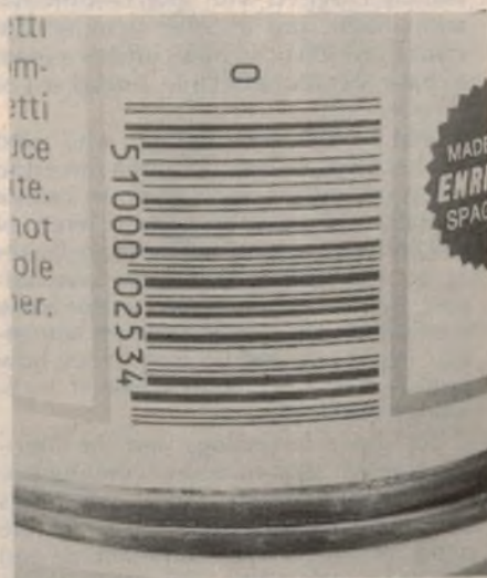
The Universal Price Code symbol identifies the manufacturer and the product by a numerical code. The store computer has information on the price and inventory of each item in its memory, ready to be used by the POS terminal.
