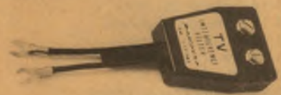
A typical high-pass filter intended for use with TV receivers using 300-ohm ribbon. It attenuates signals below about 45MHz.
