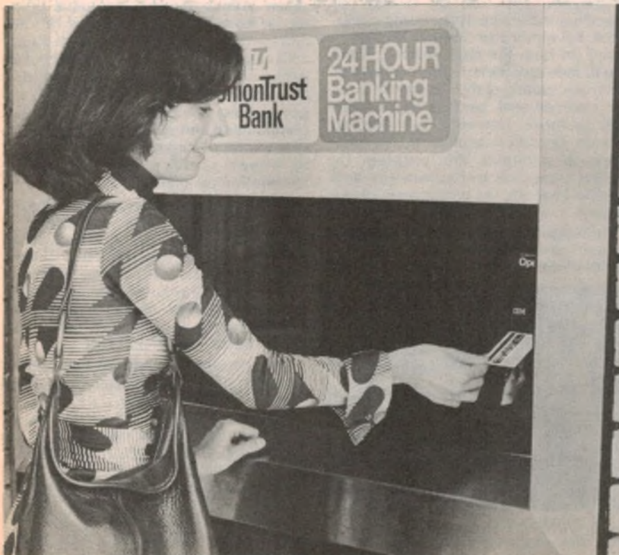
This computer terminal permits bank transactions 24 hours a day. The customer can withdraw cash, make deposits, and transfer funds between accounts.
