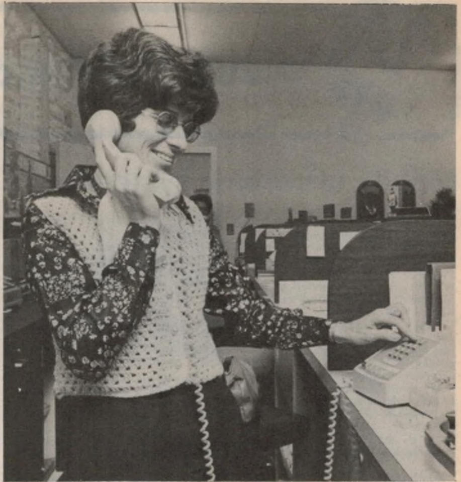
What appears to be a telephone is actually much more. It is also a computer terminal located in a small branch office of a large metropolitan bank. By dialling certain codes, the teller can connect directly with the bank's main computer to get information on balances, deposits, and withdrawals. Incidentally, the computer answers the coded requests in English.
