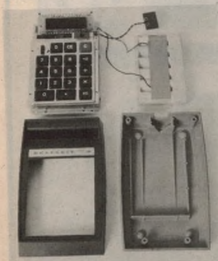
Above: the almost-completed kit, just before final assembly into its case. View at right shows the assembled main logic board, together with the plug-in keyboard and LED display.
