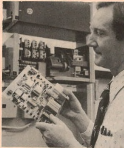
Bell Labs supervisor Ron Trupp inspects a message board from the Bell System's new recorded message machine. The machine is the first to make practical use of magnetic bubble memory devices.
