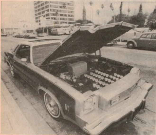
Above: a surprise for most mechanics. Powerful 180V tri-polar lead-cobalt battery system delivers more than twice the energy per pound of lead-acid batteries. Above right: Aronson and Transformer 1 at a recharging station. Bottom right: Transformer 1 in traffic. Vehicle has a similar appearance to conventional cars.
