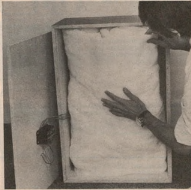
The inside faces of the enclosure are not padded but the internal space should be occupied by "Innerbond" or other similar filling. Cut a 70cm strip, 3 metres long, roll it from both ends like a scroll and stand it on end as shown, being careful not to dislodge the connecting leads as you push it in.
