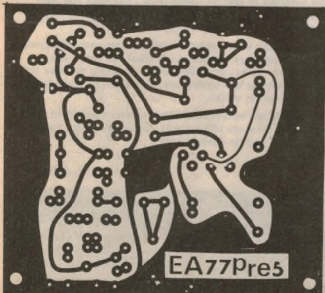
Here is an actual size reproduction of the PC board pattern.
