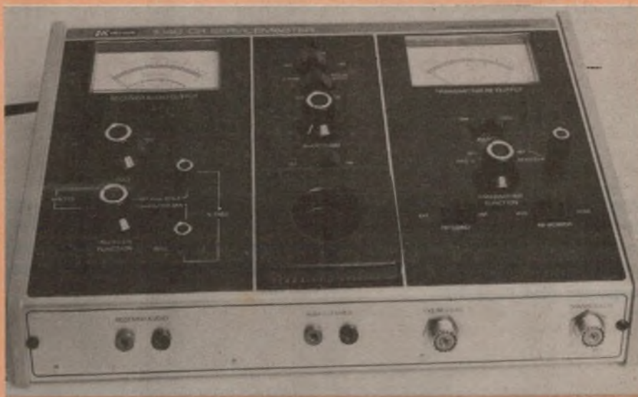
The B&K-Precision 1040 CB Servicemaster. The panel on the left has predominantly to do with testing the receiver's audio system, measuring power out and distortion. On the right is the transmitter test panel; RF power output and SWR. The audio oscillator in the centre provides single tone and two-tone output, as an electrical and an acoustic signal.
