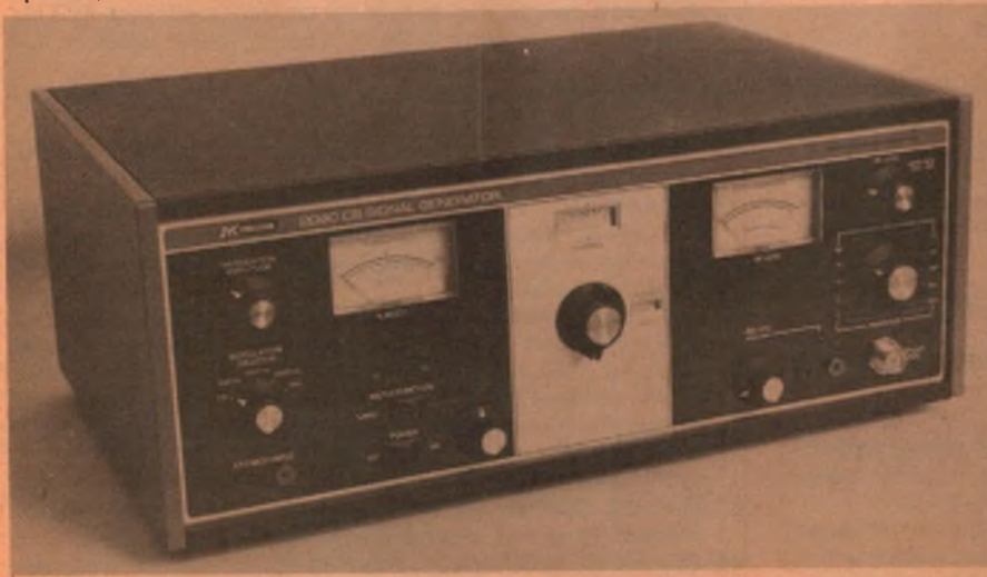
The B&K-Precision 2040 signal generator is intended expressly for servicing 27MHz CB-style transceivers. It provides output on 50 channels each 10kHz apart to a frequency accuracy of .0005%, with a offset facility of \pm 5 kHz. Leakage is very low and the attenuator is calibrated down to 0.3 \mu V. For IF alignment, there is an in-built crystal controlled oscillator.
