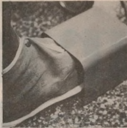
The safety foot switch showing the protective hood designed to prevent accidental operation.
