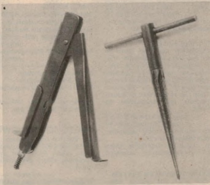
A tapered reamer and a sheet-metal nibber are useful tools for this project.
