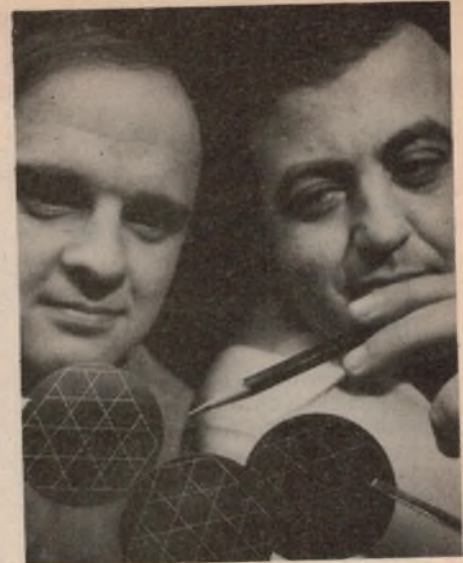
GE researchers Dr Thomas Anthony (left) and Dr Harvey Cline show new wafers made by thermomigration technique. The new technique promises to reduce fabrication temperatures and increase yields.
