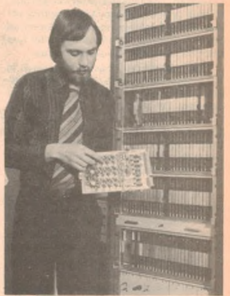
Marconi engineer, Mr Paul Batho, displays one of the 96 shift register boards making up the field store.
