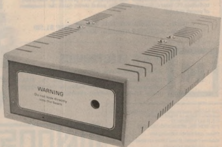
Two A & R-Soanar PC1 instrument cases were used to house the laser tube and supporting electronics. Cases are strapped together using aluminium brackets.
