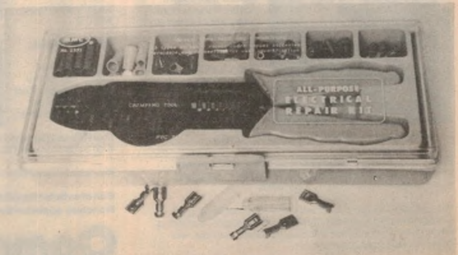
This crimping kit plus the Utilux connectors helps make rugged and reliable connections to the bridge rectifier, main filter capacitor and mains switch.
