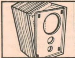
3 Wrap sides of case around baffle board.
