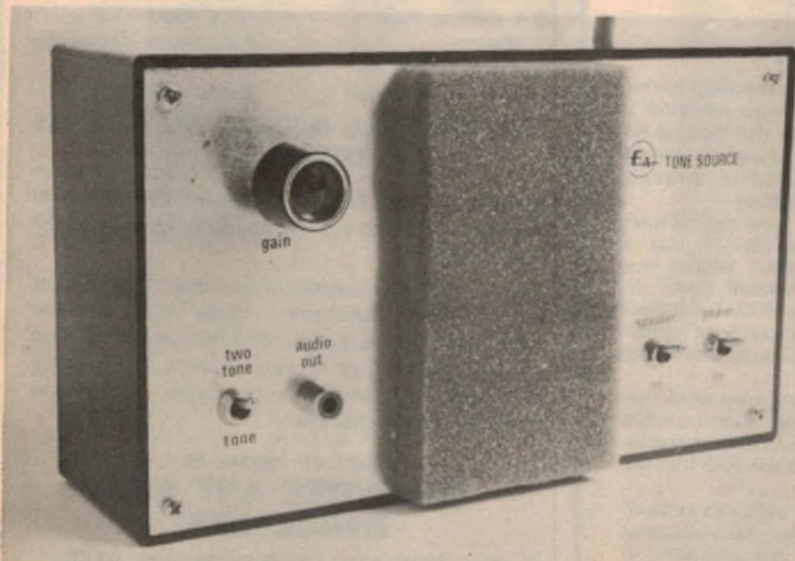
The completed prototype provides either a single 1000Hz tone or a 500/2400Hz two tone signal. Coupling may be either acoustic or electrical.
