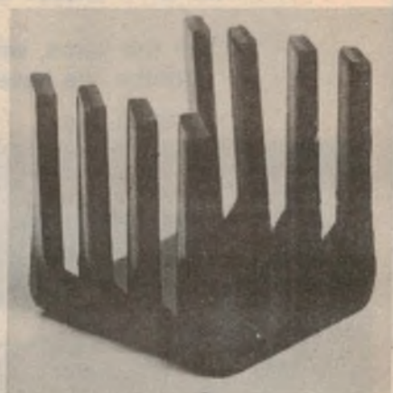
Redpoint TV4 heatsink. Thermal resistance is 17^\circ\text{C/W} .
