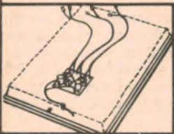
1 Screw the crossover networks to the baffle boards.
