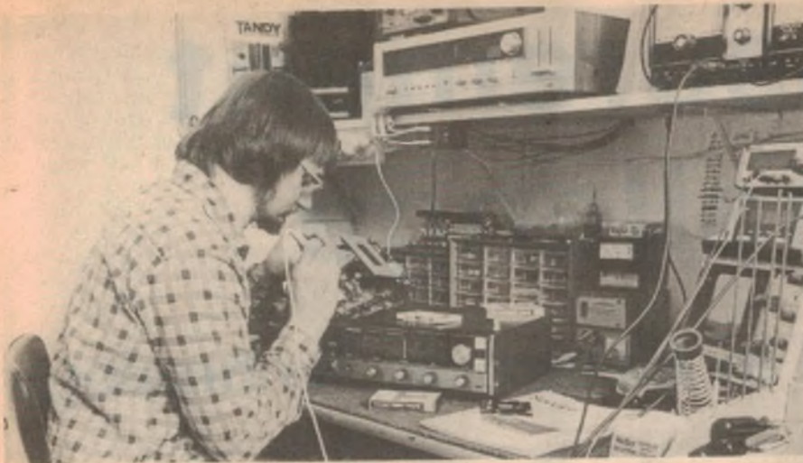
One of several well equipped booths which form the service section of the quality control department. In this case the technician is working on a cassette tape deck, but the next job may involve the output stage of a transceiver.
