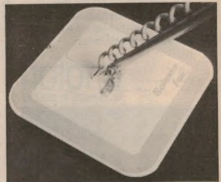
The search coil supplied with the 28-181 kit. It is fitted with an electrostatic shield on the underside.
