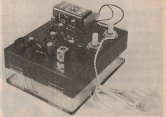
The simpler version of the detector, built on a plastic chassis. Note how the search coil is wound on the clear plastic portion of the original box. Sticky tape holds the coil in place and the two halves of the box together.
