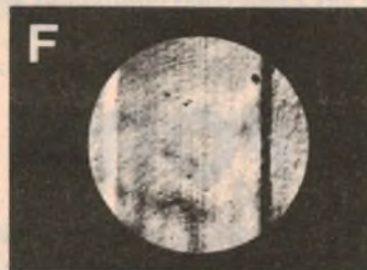
Elliptical Stylus caused excessive wear after 100 playings — magnified 12000 times
