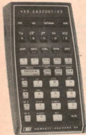
The now famous HP-65 programmable pocket calculator. Magnetic cards enable it to use pre-recorded programs.
