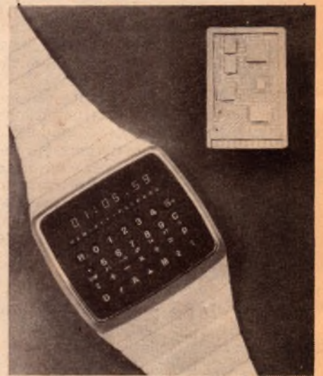
IC chip (upper right) is brain of HP-01 Computing Time Instrument.
