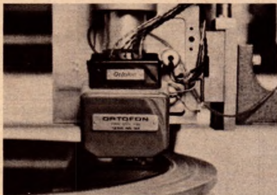
Ortofon professional cutter head type DSS 732 in action.
