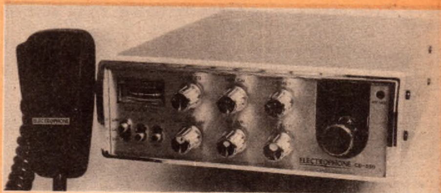
Above, the Electrophone CB-550 SSB/AM transceiver and, below, the CB-590 base station. It would appear that both use much the same PC board assembly, hand wired in each case to the appropriate peripheral controls, metering and access sockets.
