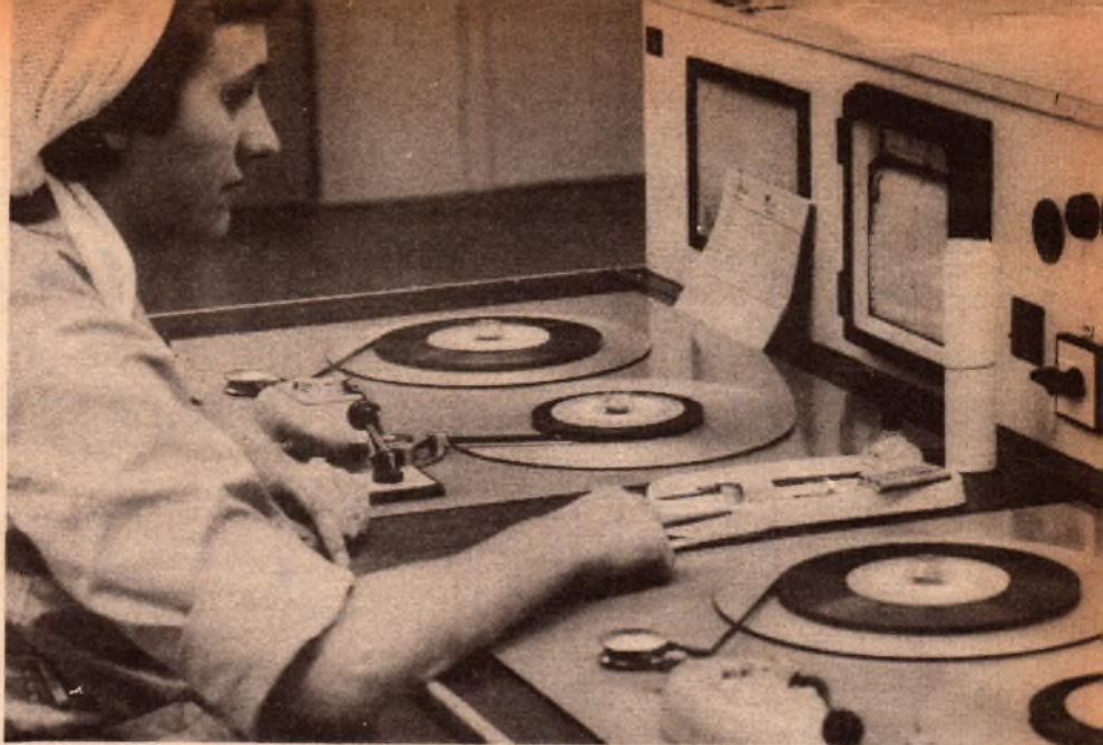
Newly spooled tape from the slitter is checked on special equipment to ensure that it conforms to standard. Later, it will be cut into commercial lengths, fitted with coloured leaders and spooled into the familiar reels and cassettes.
