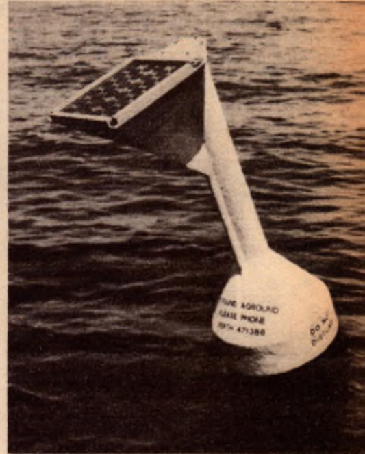
Solar panels were used to power drifting buoy transmitters as part of a recent CSIRO marine research program.
