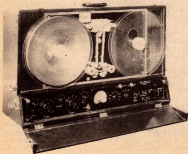
One of Arthur Smith's more recent sound recorder designs: a fully transistorised portable magnetic recorder using 17.5mm film, produced in 1961.
