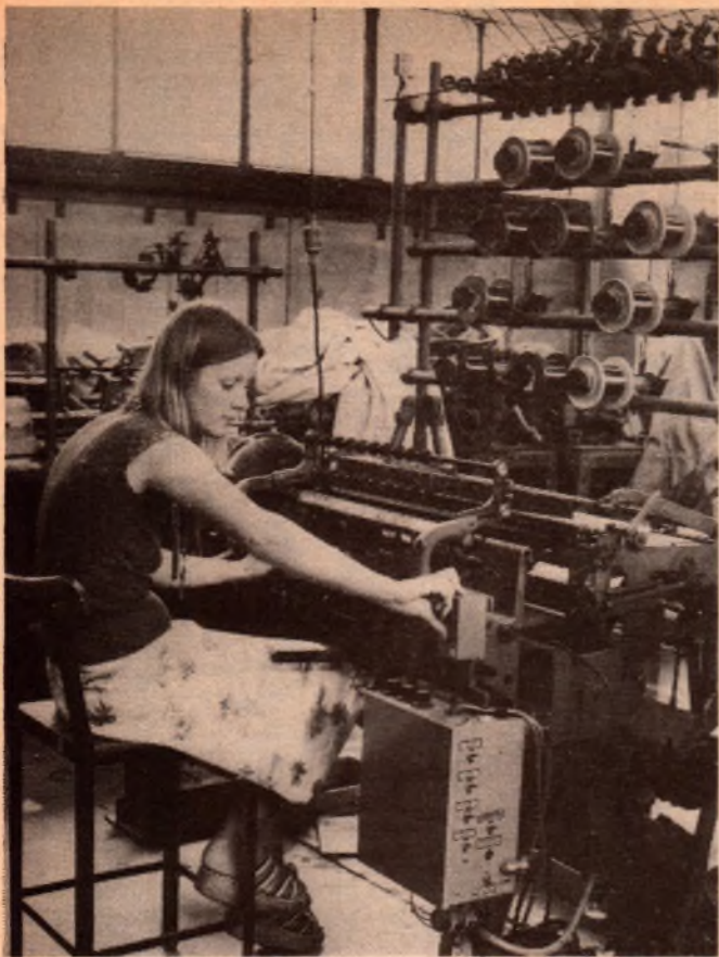
Pictured above is the older method for winding transformers. Miss Barbara Dickson hits the button on the "stick" winder to wind 10 coils simultaneously. Meanwhile, below, Mrs Vicky Tsiganos works on the newer method with the large bobbin winder. Transformers now account for about 20% of A&R sales.
