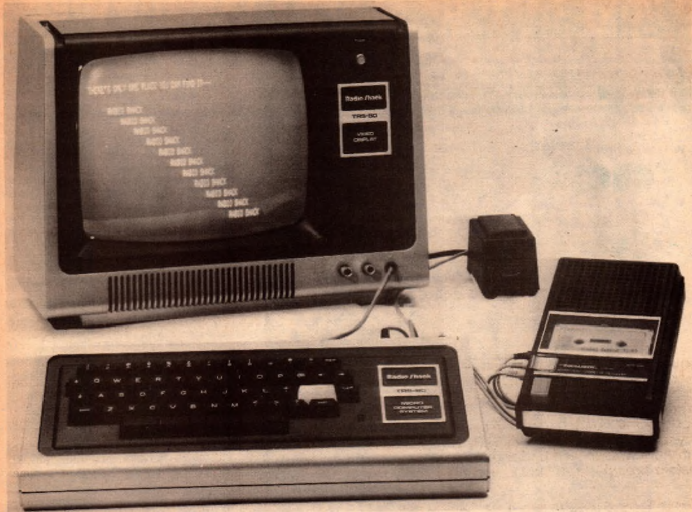
A closeup of the complete TRS-80 system. The computer itself is inside the keyboard unit; the TV monitor and cassette recorder are quite conventional. As you can see, there are no highly technical controls.
