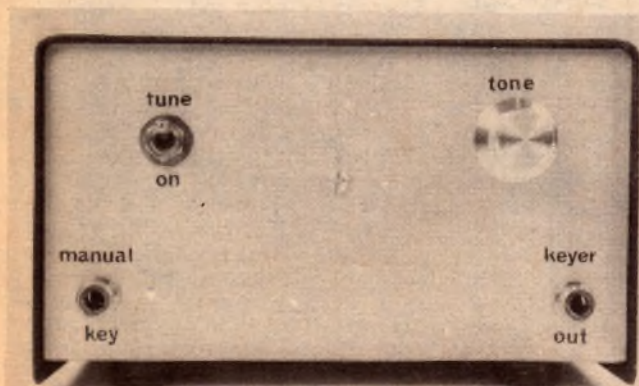
The rear panel of the Electronic Morse Keyer. RCA sockets were used for the "manual key" and "keyer out" input/outputs.
