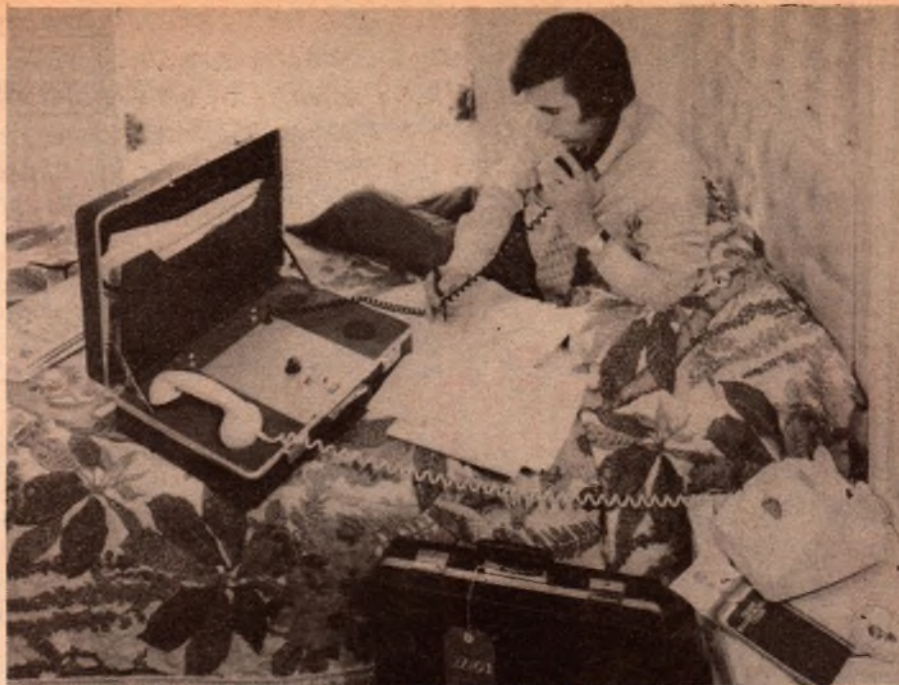
One obvious use of electronic speech synthesis units is in voice scrambler circuits for security applications. This British device, known as the "Privateer" is able to scramble and unscramble telephone conversations.
