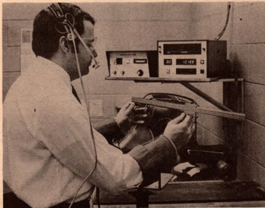
Paralleling the development of machine speech systems are machines that can recognise spoken words. Above is Threshold Technology's Voice Data Entry System (VDES), a voice recognition system that enables data to be entered verbally into a computer.
