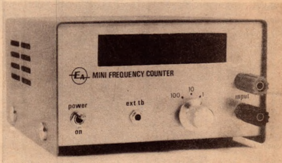
Provision for external timebase and 5-digit readout are features of the design.
