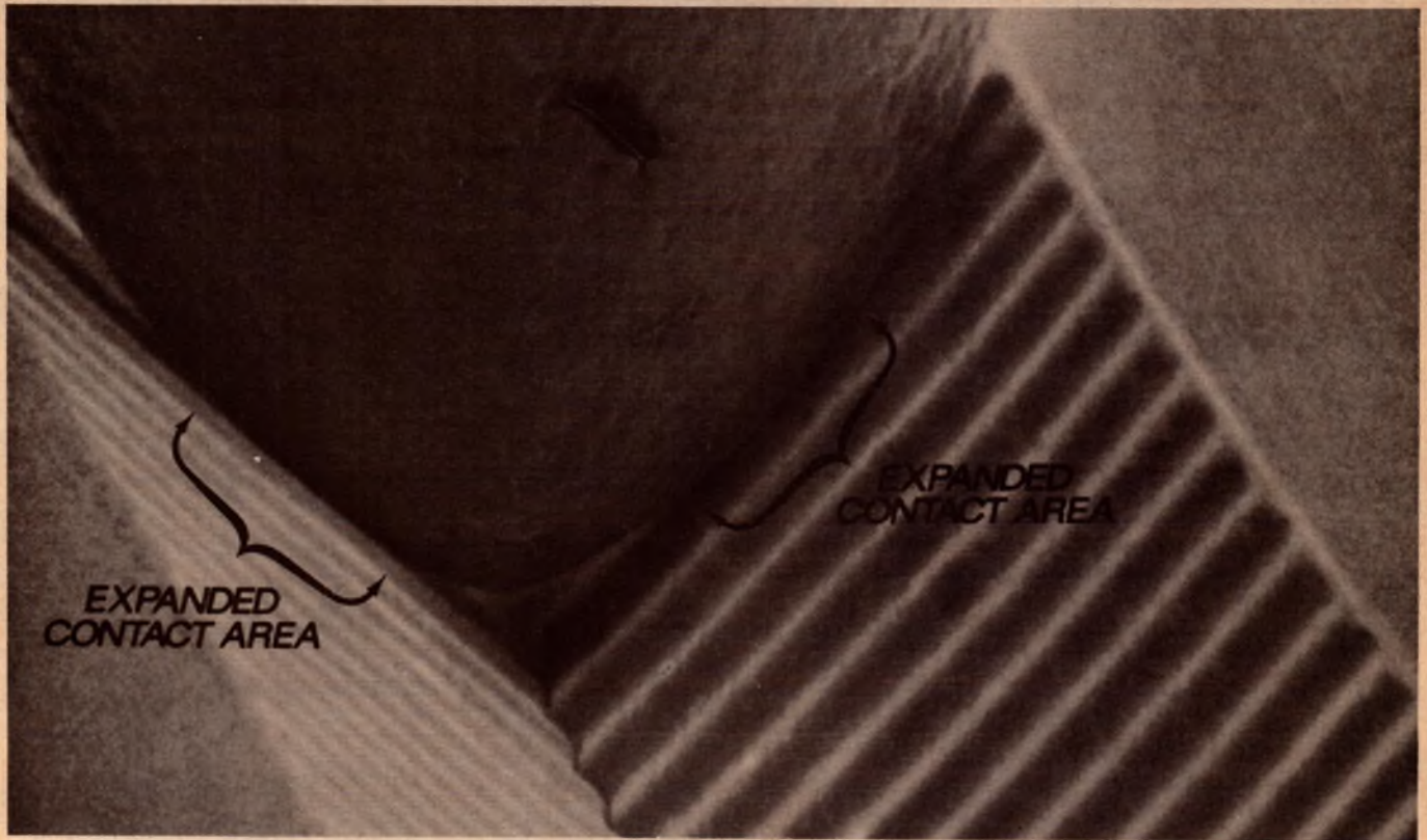
Scanning Electron Beam Microscope photo of Stereohedron Stylus; 2000 times magnification. Brackets point out wider contact area.
