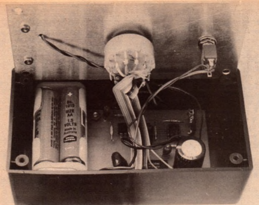
View inside the completed Utility Timer. Take care when mounting the PC board to ensure that the large electro does not foul the off/start switch.
