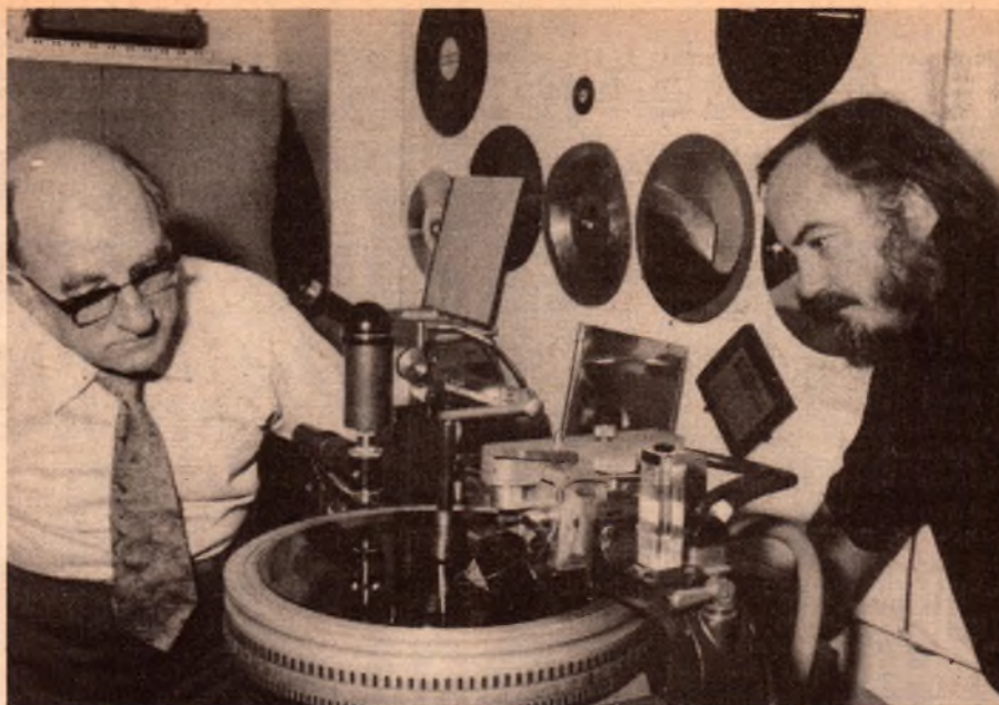
Production engineers Max Hull (left) and Bill Hawtin (right) watch the first test cut being made. The lathe is the Astor Record Company's Neumann ZT32S, fitted with an SX74 cutting head.
