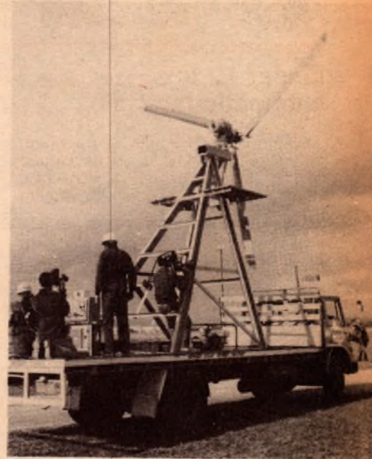
Prototype 5kW wind-powered generator undergoing tests at Edinburgh RAAF Base, South Australia.
