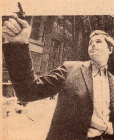
An engineer tests the acoustics of the new Oslo Concert Hall by using a pistol as the sound source.
