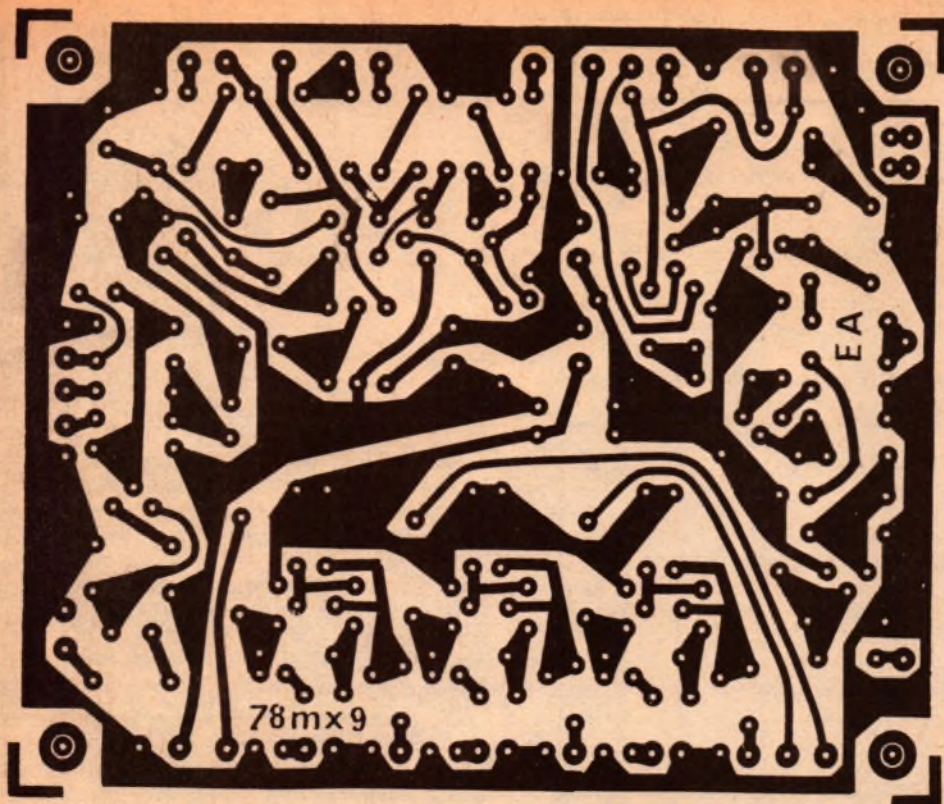
Here is the PCB pattern for the mixer, reproduced actual size for those who may care to produce their own board by tracing or photography.
