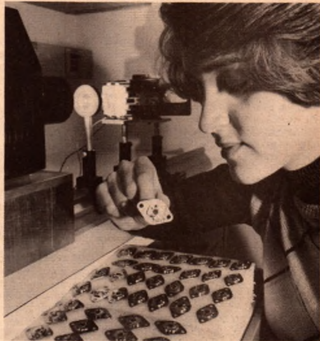
Researcher John Hughes examines an array of plastic lenses used to focus the Sun's energy onto silicon solar cells. RCA's experimental 300W system continually tracks the Sun, and could significantly reduce solar energy costs.
