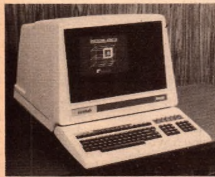
The Ramtek 6200A "Colorgraphics" terminal features full colour graphics and alphanumeric capabilities, teletype compatibility, a 32cm colour monitor, and eight selectable colours.
