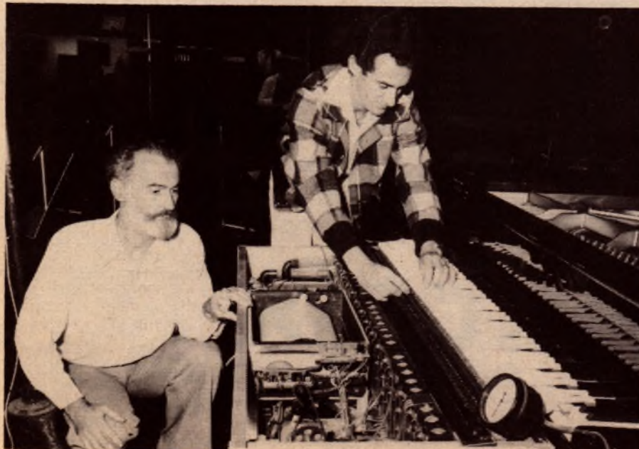
Denis Condon (left) and Peter Phillips at work on the Vorsetzer prior to its Opera House performance last June. Photo clearly shows the aluminium fingers.
