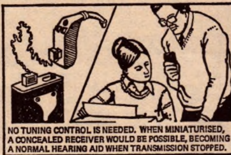
NOW CSIRO, WITH THE NATIONAL ACOUSTIC LABORATORIES, HAS DEVELOPED A NEW METHOD OF SHORT-RANGE WIRELESS TRANSMISSION USING AN F.M MAGNETIC INDUCTION FIELD, TRANSMITTED AND RECEIVED BY SMALL FERRITE ROD ANTENNAS.
