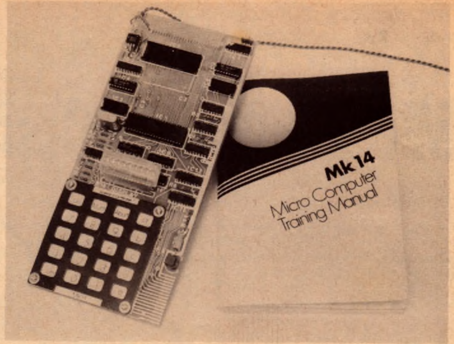
The Mk 14 Micro Computer and its accompanying Training Manual. We recommend that a heat sink be fitted to the regulator IC, as this can become quite hot.
