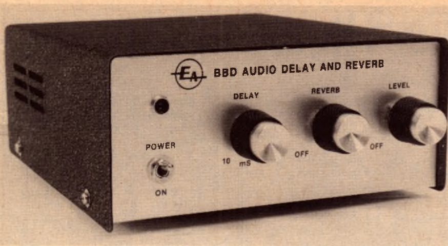
View at left shows the completed prototype, housed in a standard metal case. The amount of delay is variable from 10ms to 50ms.
