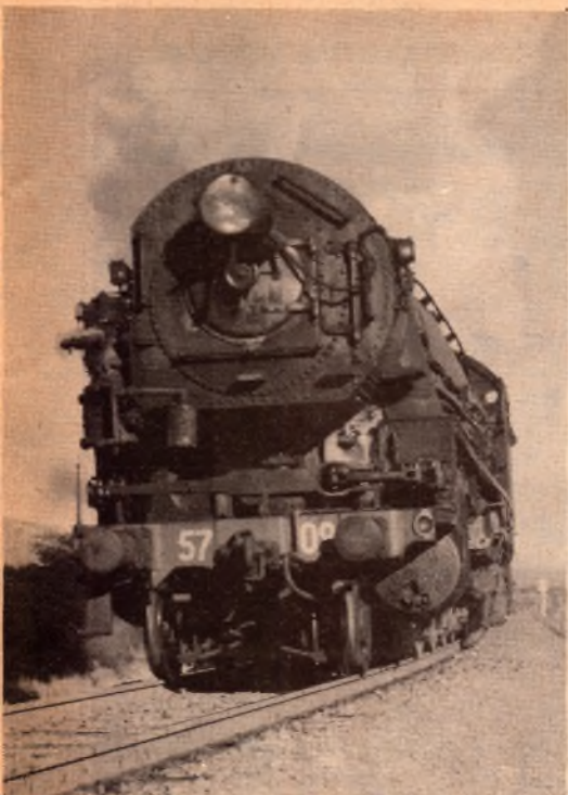
Perhaps things will never be quite like this again, but we couldn't resist publishing the above picture of one of the old D57 "Mountain" type locomotives. The D57 weighed 230 tonnes and was one of the most powerful steam loco classes built in Australia.
