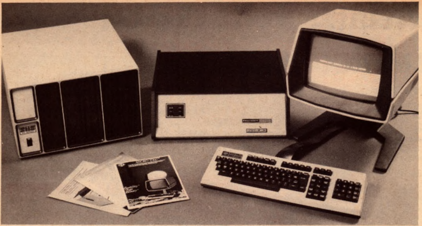
Here the Heath H-11 is shown with an SMS dual floppy disc unit and a Micro-Tec model 70 video terminal. The H-11 runs a great deal of the software written for Digital Equipment PDP-11 computers.
