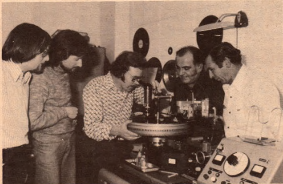
Frank Hulbert (centre) sets up the microscope to inspect the grooves of a direct-cut disc which has just been completed at the Astor plant in Melbourne. Anxious to see how it turned out are members of the Steve Murphy Quartet, who had just made the recording. (See our August 1978 issue, page 27).
