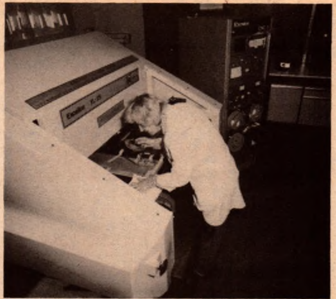
ly controlled machine which automatically — and accurately — drills holes in printed circuit boards for telephone exchanges.
