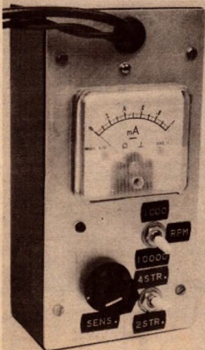
At left is the author's prototype tacho, made using parts on hand. If you are building from scratch, a larger meter and case could be used to advantage. Above is a close-up of the shielded capacitive pickup probe, partly opened.
