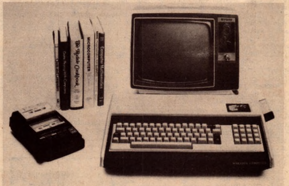
Here is the Sorcerer in a typical user situation, with the BASIC interpreter cartridge plugged in the side. The TV monitor, cassette recorder and books don't come with it for the price quoted — they're extra!
