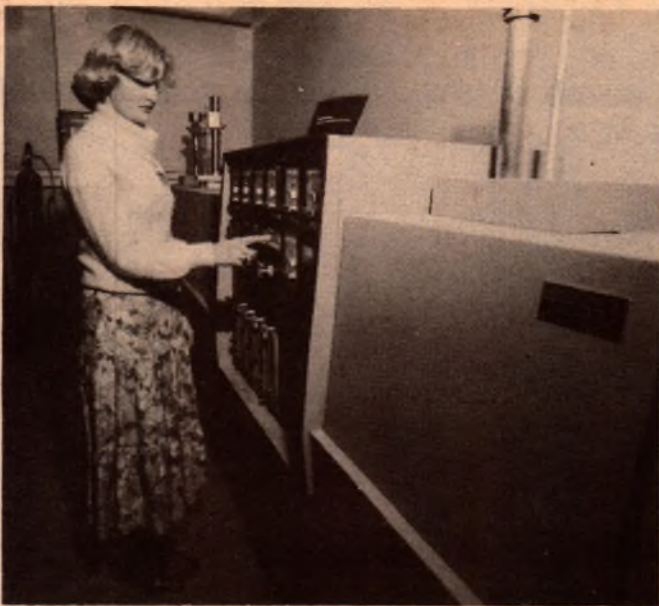
Above: Labs staffer Cheryl Crarey indicates the control panel of a bank of furnaces which fire thick film conductors at temperatures up to 850°C. View at right shows Tech. Assistant Eta Horvath setting up the Lab's new $70,000 numerical-
