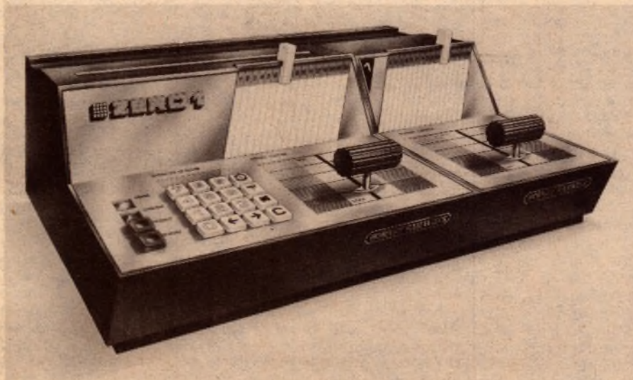
Artist's concept of Hornby's Zero One model train controller. View shows the master control unit together with one of the slave control units.
