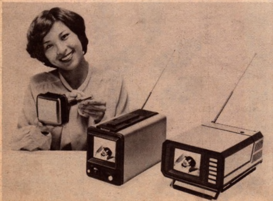
Single-gun, single-beam colour TV tube without shadow-mask (left), and two 10cm colour TVs using the tube.
