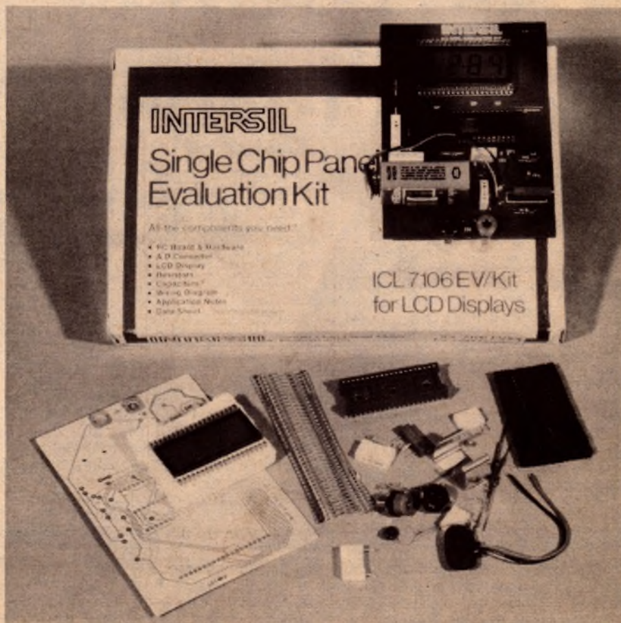
This photograph shows an assembled kit, and the components required to construct a second kit. Note the battery clamp.
