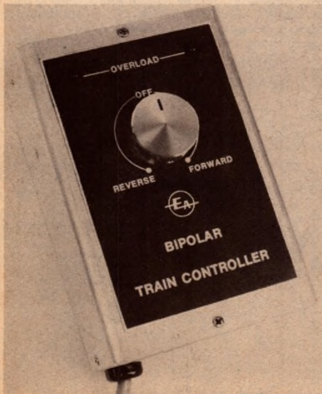
The neat appearance of the prototype can be seen in this photograph. One or other of the LEDs will light in an overload condition.
