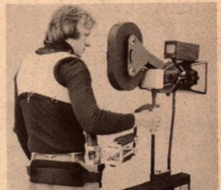
The Steadicam system features a specially designed high-intensity monitor which permits viewing in all ambient light conditions.
