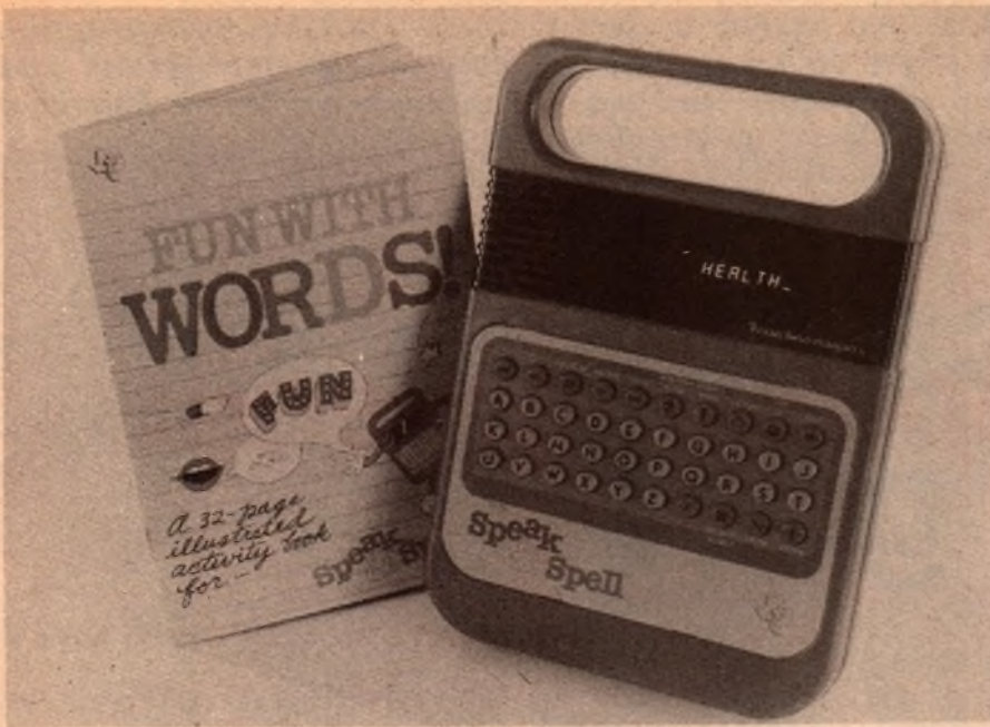
Speak & Spell comes with a 32-page activity book. Unit reads out its 200 words randomly for various spelling exercises selected via the keyboard.
