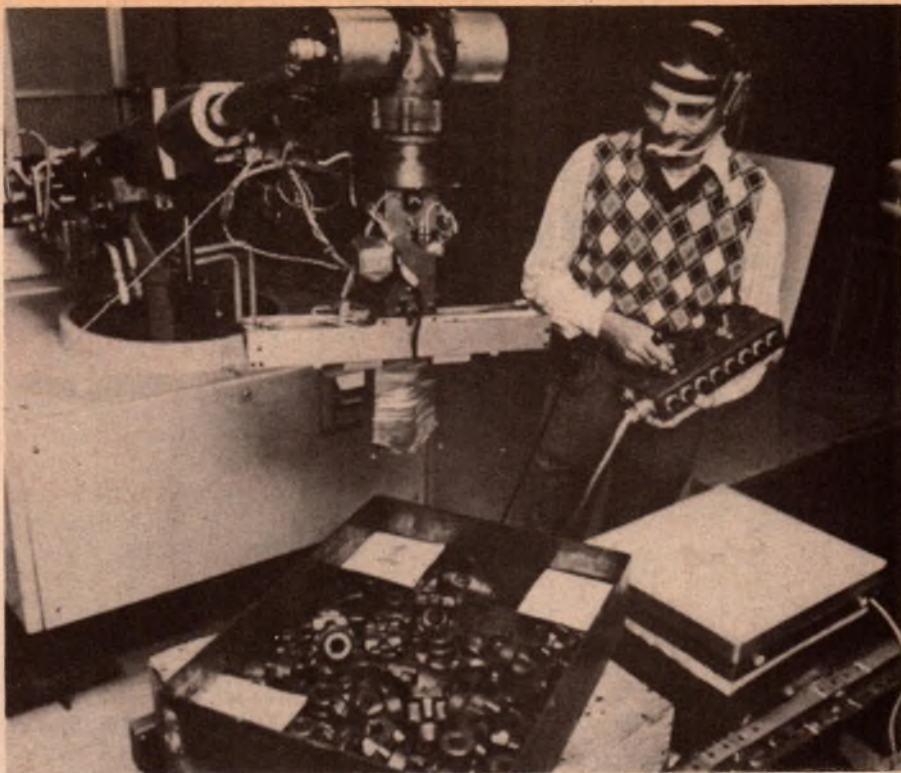
An operator trains the system to identify and pick up objects.
