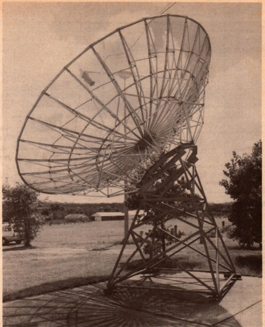
ABOVE & RIGHT: Two views of the 5-metre parabolic dish antenna.
