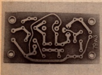
A printed circuit board. The copper tracks form the wiring connections.
