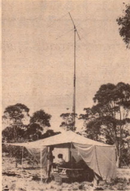
The Wagga Amateur Radio Club's 10m and 15m tent on Mt Granite for the John Moyle Memorial National Field Day. The aerial on top of the mast is a 10m quad. (See story, page 110.)
