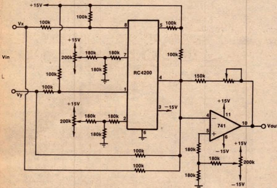
If you wish to keep a continuous record of DC power levels using a chart recorder, it is best to plot voltage squared, as power is then given by the area under the graph. In an experiment at Hartley College of Advanced Educa-
