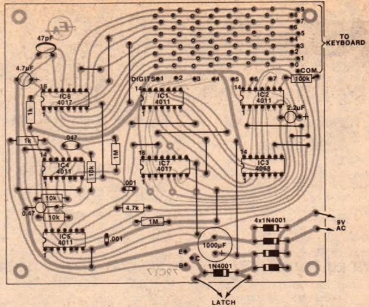
Use this overlay diagram in conjunction with the circuit to assemble your unit. Don't forget to add programming links to make up the 7-digit code you require.
