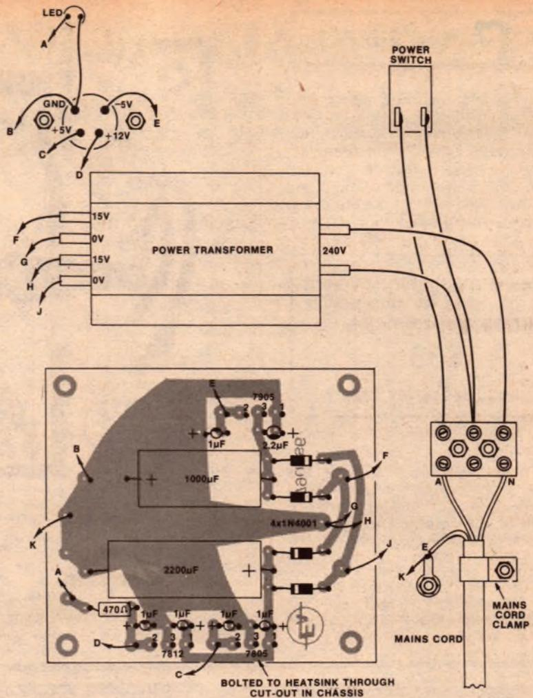
Follow this diagram and the photograph below for easy assembly of the power supply.
