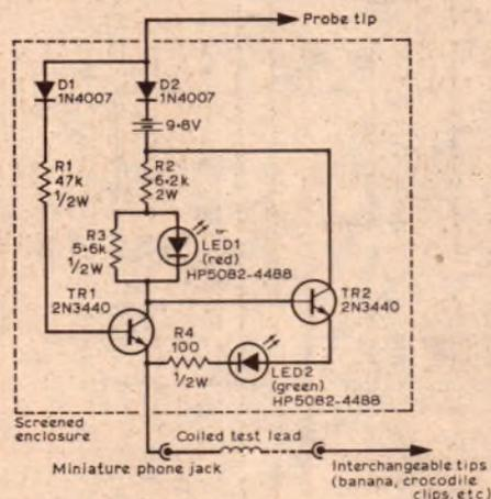
two points between which there is continuity but no potential difference, current from the internal battery forward biases TR2 and turns it on. The green LED then lights, but the small base current is not sufficient to cause
