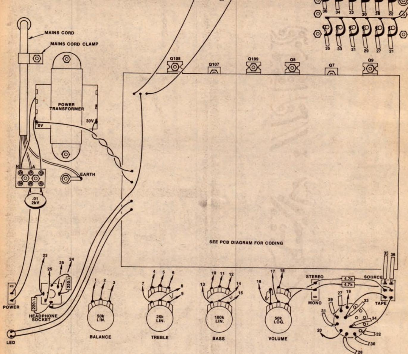
Use this diagram in conjunction with the PCB layout to complete the amplifier wiring.
