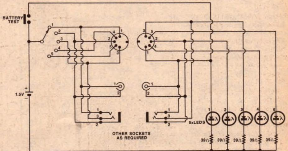
The design presented here is powered by a single dry cell and needs no power switch since the act of plugging in a cable completes the circuit. The battery test button is operated momentarily before using the device. LED No 1 should light, indicating that the battery is OK.
