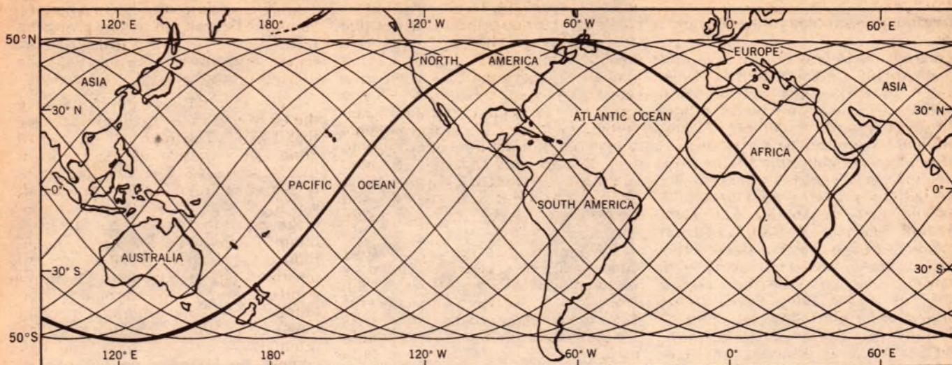
Skylab's angled flight path ranges 50 degrees above and below the equator. If the Earth didn't spin, Skylab would trace out the same path on every pass. Instead, the craft traces out a series of different
