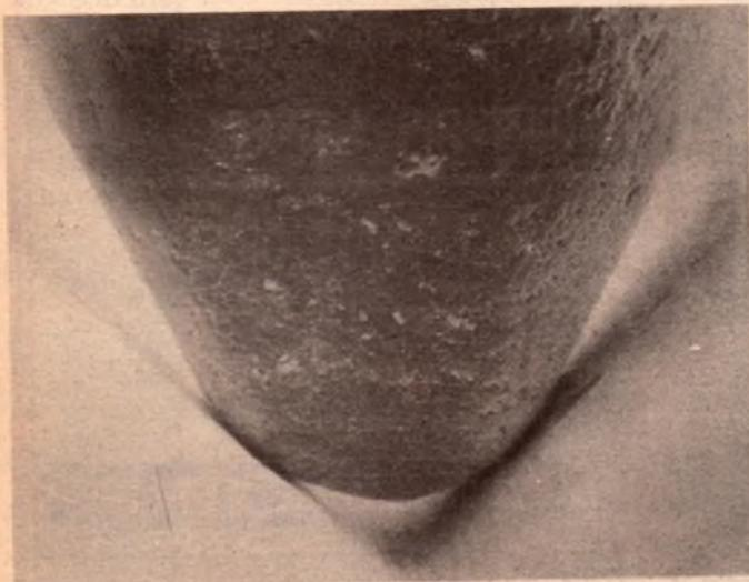
Fig. 1: A conventional spherical styli having a tip radius of 0.7 mil resting in a groove. Note the limited contact area, which has to support the total playing weight.
