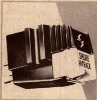
**M91ED** ... excellent trackability at a lesser price. Shure Hi-Track has a smooth 20-20,000 Hz frequency response, 3/4 to 1 1/2 grams tracking force and an output voltage of 5.0mv per channel. Nude mounted diamond stylus tip.
