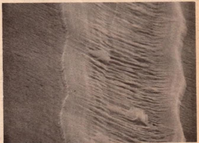
Fig. 6: A surprising observation was the effect of playing a disc when moistened with water. Far from lubricating the surface, it actually produces a tearing effect as shown.
