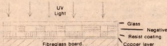
UV light passes through the clear areas of the negative and sensitises the Resist. Black areas on the negative prevent the UV light from reaching the Resist. During development the unsensitised areas of Resist are removed, leaving the acid resistant sensitised image.
