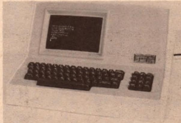
and lower, conversational mode or page edit mode, full or half duplex, set baud rate (31 speeds available from 50 to 38,400 baud), and shift mode normal or inverted. Another 22 codes control the CT-82's responses to control characters, and their display or non-display.
