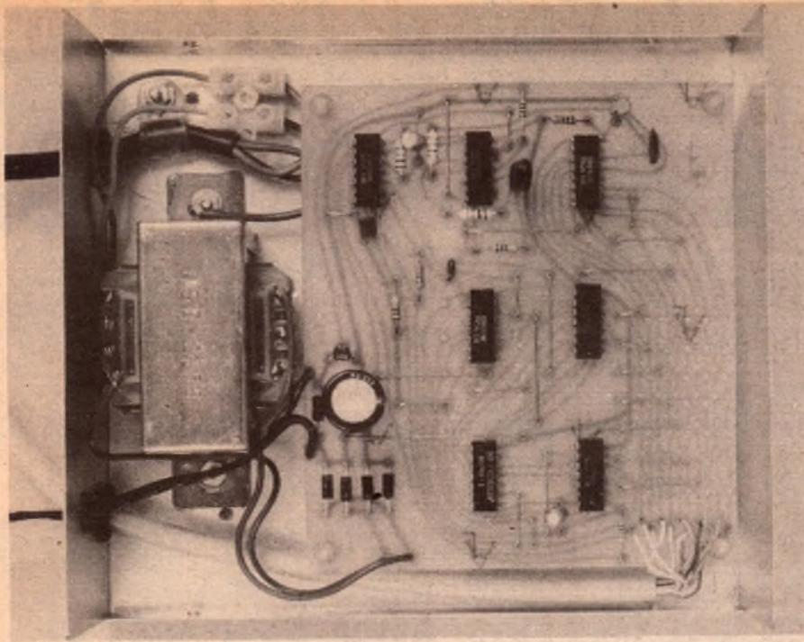
Inside the completed electronic combination lock. Programming links have been added here to give a 0123456 demonstration code.
