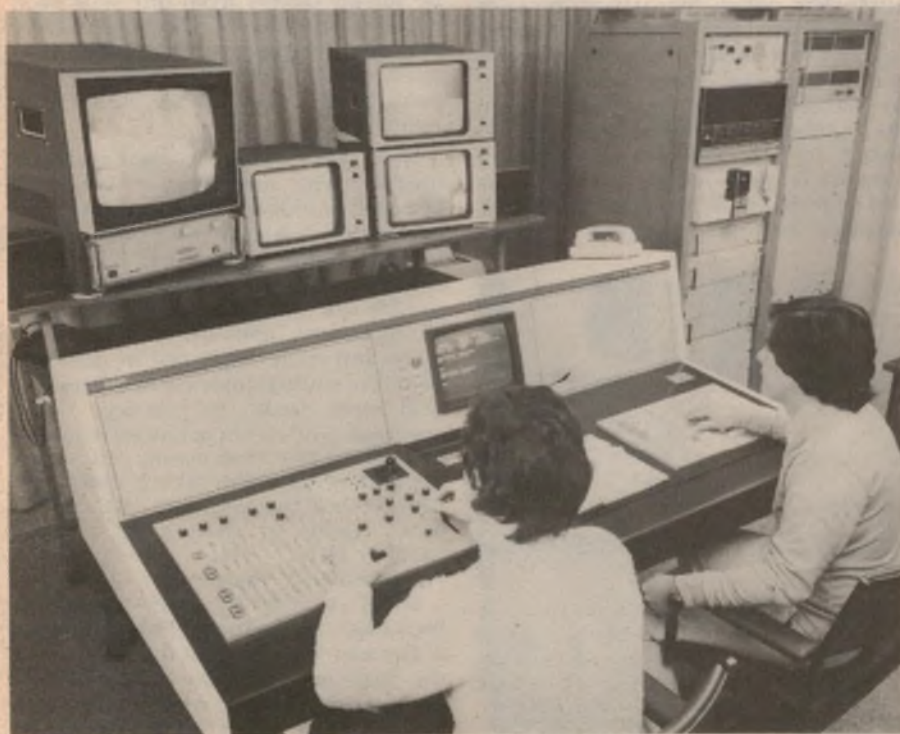
Students at the control console of the School's computer controlled videotape editing system. Based on a Nova minicomputer visible in the rack at right, the modified Central Dynamics system was supplied by Philips.
