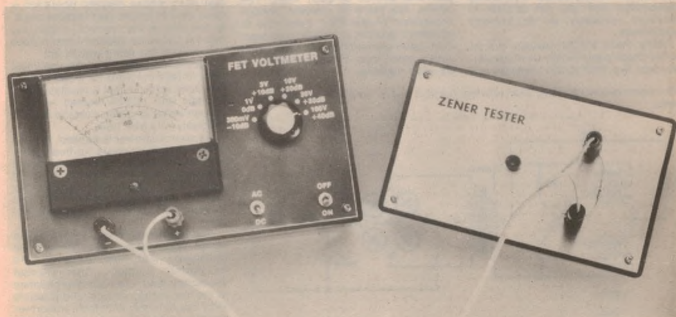
You can readily identify those small zener diodes with our new Zener Tester, and also check breakdown voltages of transistors.
