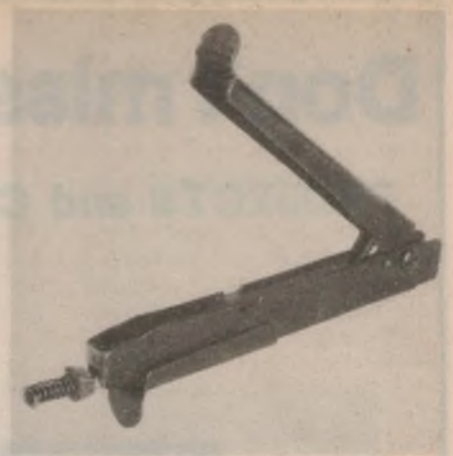
A nibbling tool is used for making cutouts in sheet metal panels.
