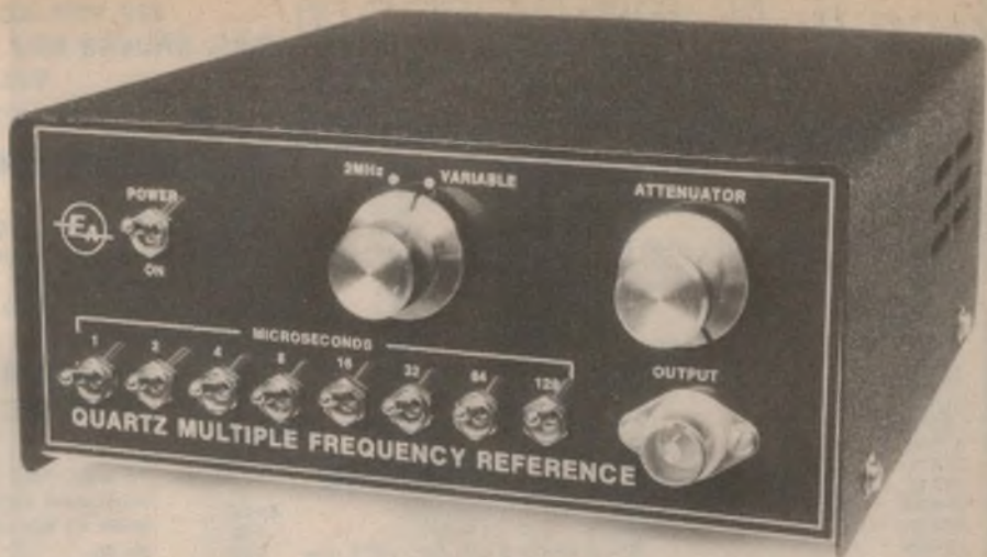
The prototype was built into a standard metal case. Eight toggle switches and one rotary switch give accurate square wave frequencies from 4kHz to 2MHz.
