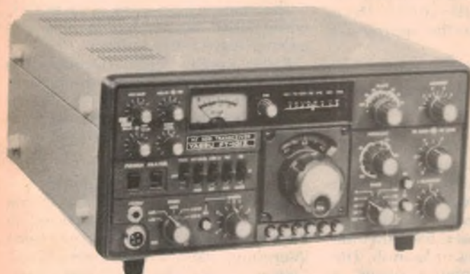
The Yaesu FT101Z. Note the linear scale above the main dial, which replaces the digital readout in the FT101ZD. One turn of the knob gives about 17kHz shift on the main tuning dial.
