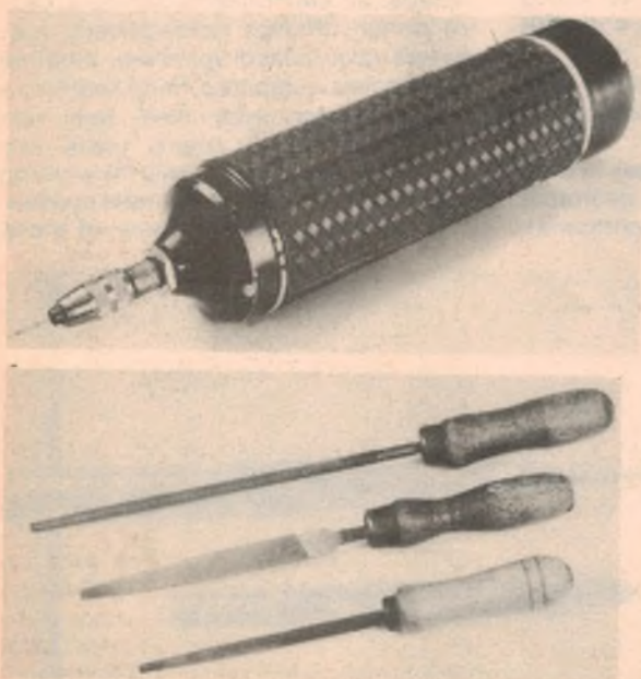
This file set includes round, flat and triangular files.
