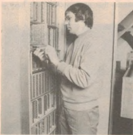
Myk Fairhurst at the electronics cabinet, which contains close to 8000 ICs on 100 PC boards. (Photo by Warren Webb.)
