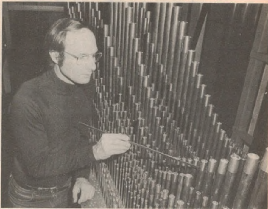
Builder Ron Sharp shown tuning pipes in the main or "Hauptwerk" division of the organ. (Photo by Don McMurdo.)
