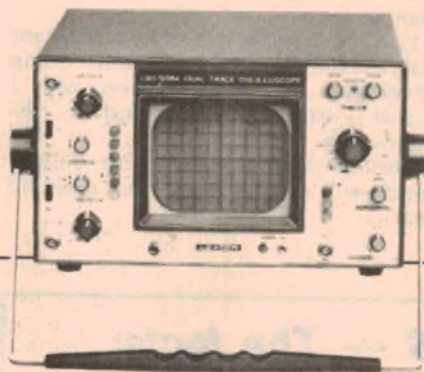
Model LBO-508A. A dual trace oscilloscope with 20MHz bandwidth and 10 mV/cm sensitivity. Multiple mode functions. 130 mm CRT produces a bright, sharp display. Display offers chop, alt., add and subtract Ch. 1, Ch. 2, X-Y
