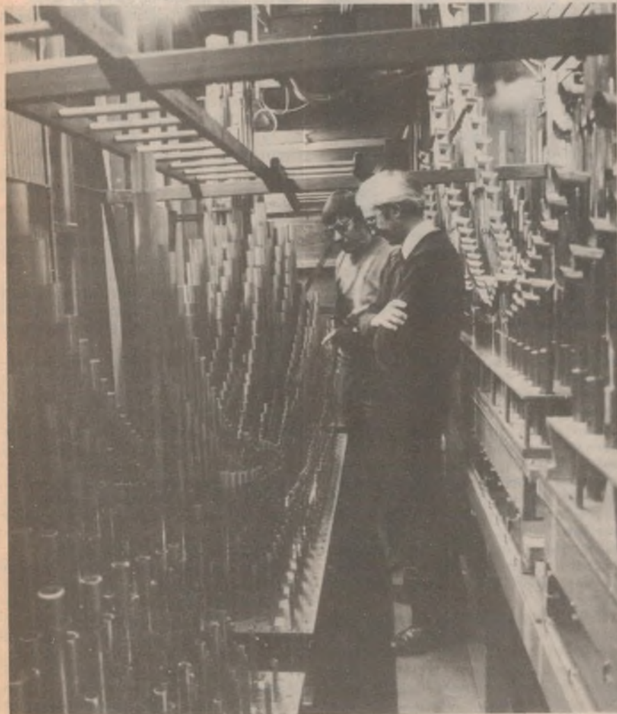
Electronics engineer Myk Fairhurst showing the author some of the pipes in the Hauptwerk division. This division alone has more pipes than most medium-sized organs. Behind us are reed pipes; in front flue pipes. (Photo by Warren Webb.)
