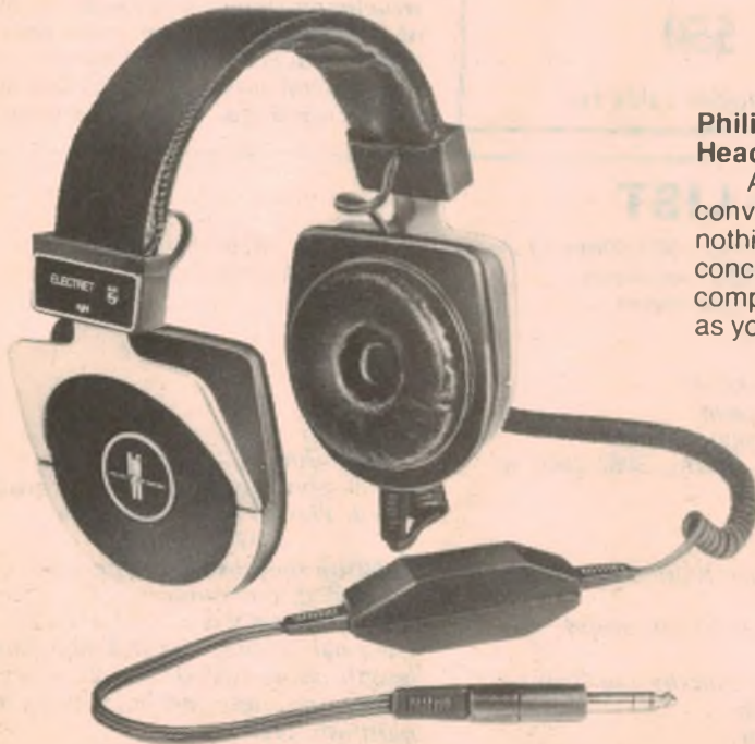
Philips N6325 Electret Headphone (Above) The electret principle embodies all the advantages of electrostatic sound reproduction, yet manages this without cumbersome weight or expensive power supplies. There is no reduction in performance, but there is a significant fall in cost.
