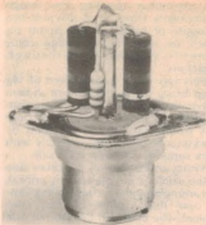
This simple dummy load was made from two 100-ohm carbon resistors mounted on a Belling Lee Socket. The third resistor was used to trim the value to exactly 50 ohms. Checked on an SWR meter it gave a 1/1 reading.
