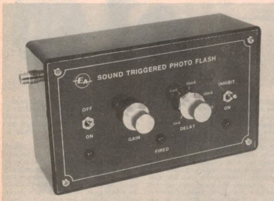
The prototype provides variable time delays from 1ms to about 120ms. The centre LED comes on to indicate that the unit has fired.
