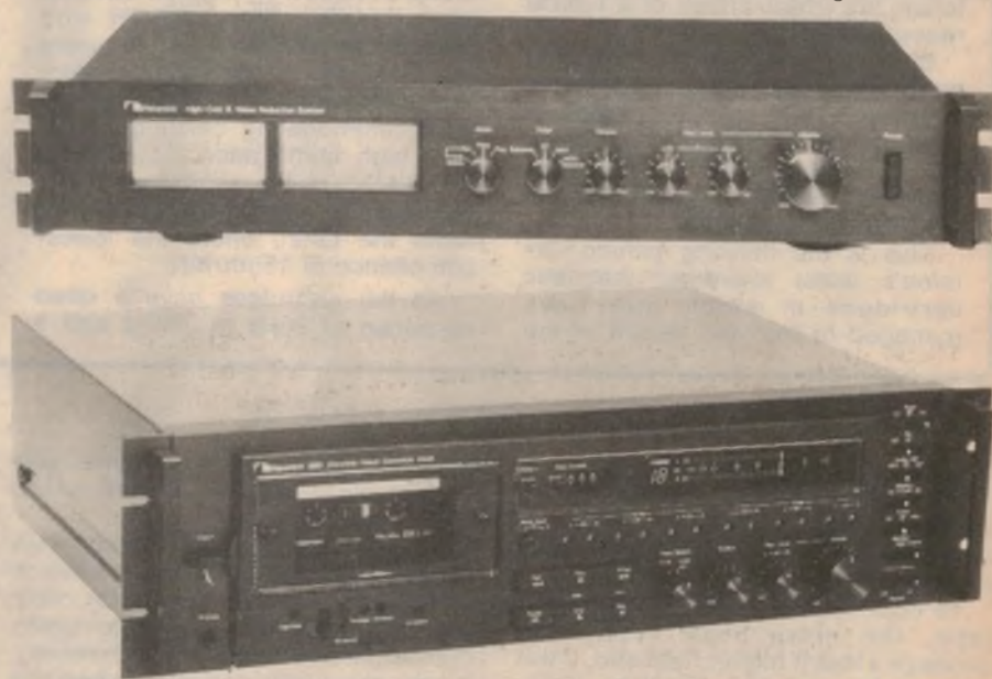
THE VERY LATEST from Nakamichi — High Com II Noise Reduction System (top) mates with a conventional, top ranking cassette deck to provide 20dB noise reduction across entire audio spectrum. Superb new model 680 cassette deck immediately above can play both oxide and metal coated tapes, and features full or half speed operation, fluorescent metering, touch controls, and both Dolby and High Com II noise reduction.
