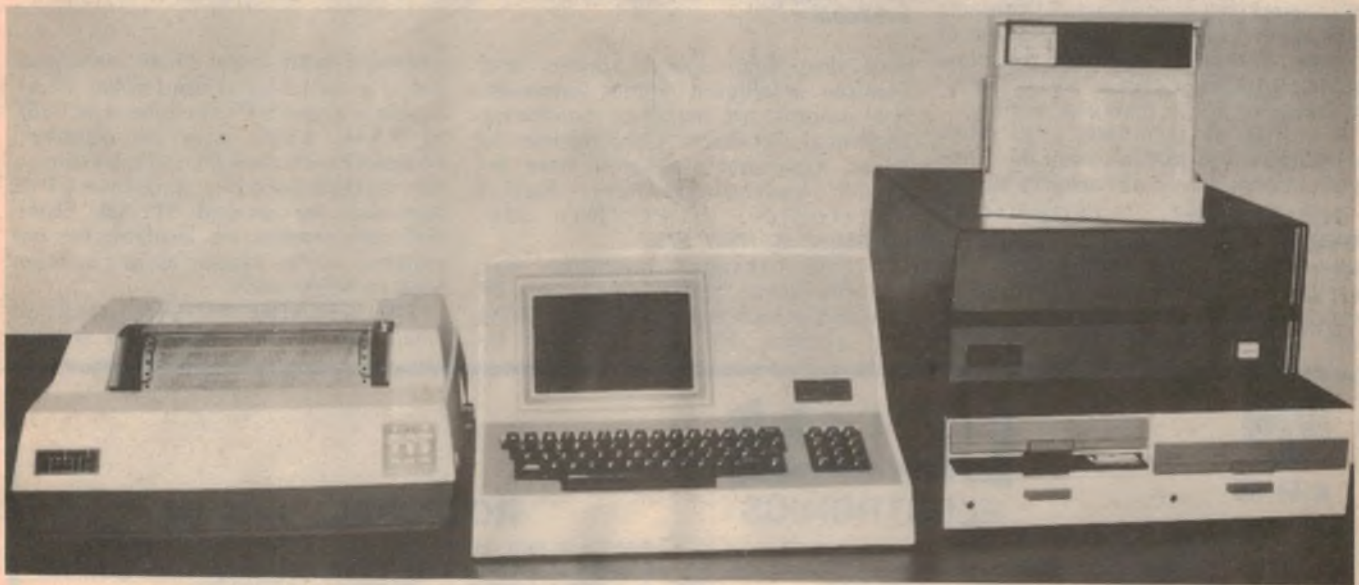
TOP: The Vector Graphic Memorte professional word processing system, based on the same firm's System B microcomputer system.
