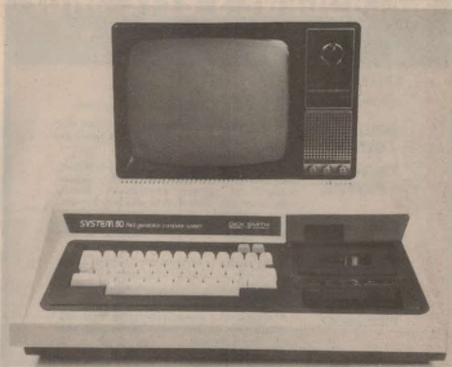
DICK SMITH SYSTEM 80: Shown here with optional TV monitor, in basic form. A recent entry in the personal computer market, it offers full compatibility with Tandy TRS-80 Level II software.
