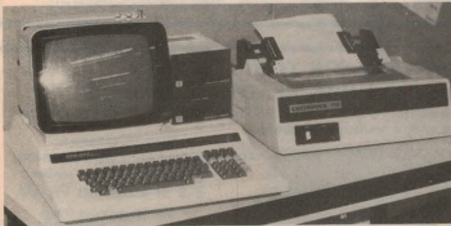
SORD M203 MARK II: This is the "bigger brother" of the M100 ACE-1 system described in the text, shown here with a Centronics printer. The M100 machine is similar, but has only one disc drive.
