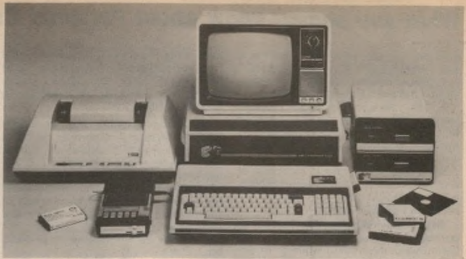
THE EXIDY SORCERER: Shown here with expansion unit, TV monitor, dual mini-floppy disc drive, cassette recorder and line printer. Also visible at front right are the plug-in ROM PAC modules.
