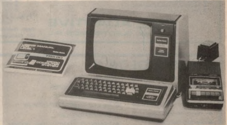
TANDY TRS-80: This is the basic 4K "Level 1" machine, which comes with 30cm monochrome video monitor, cassette recorder and power supply. It also has an extremely well-written user's manual.
