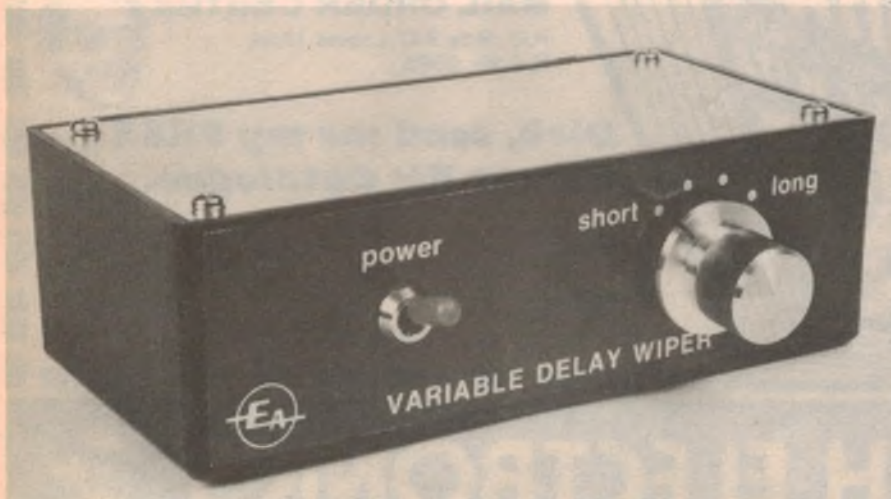
The completed prototype, built into a plastic case. It provides four switchable delay times — 3, 6, 10 and 15 seconds — and is simple to use.
