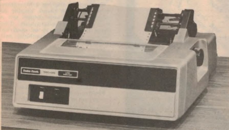
TANDY LINE PRINTER: This is the tractor-feed line printer marketed by Tandy to suit their TRS-80 systems.
