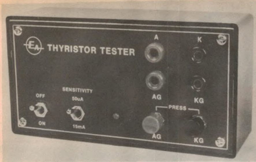
Here is the finished tester, housed in a small plastic utility box. To keep cost down, a LED is used as the test indicator.
