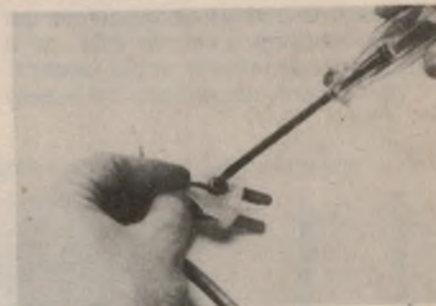
3. Tighten terminal screws firmly.
