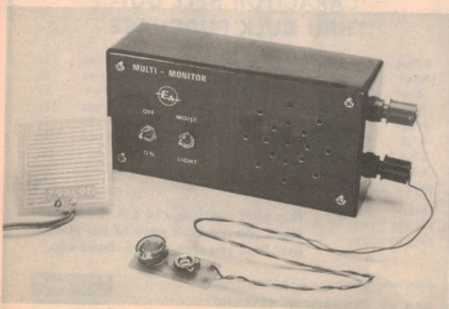
This photograph shows the complete unit with the two sensor boards.
