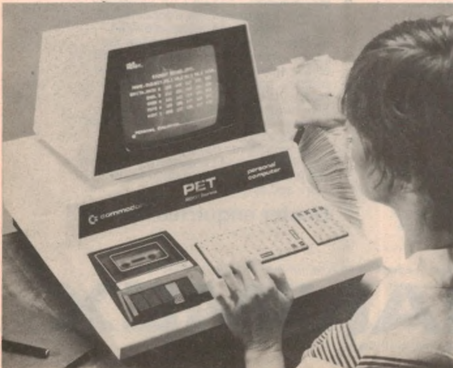
LEFT: The Commodore PET, shown in a typical file management application. Note its inbuilt cassette tape deck.
