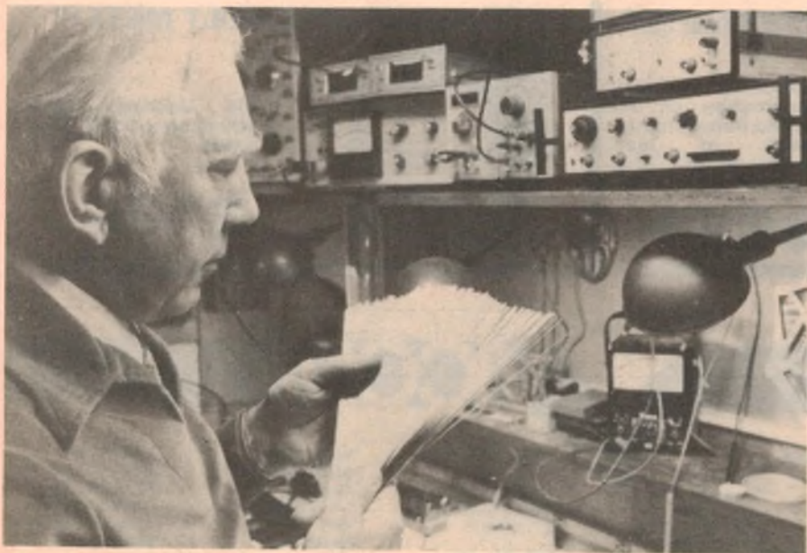
John R. Wiegand inspects a batch of specially treated wires that possess the unique magnetic property he discovered. When moved past a magnet, the wire cores shift polarities rapidly, generating strong electrical pulses of several volts.
