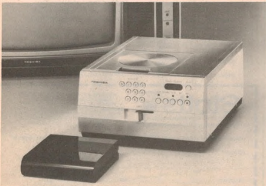
Representing a completely different approach to video cassette recording, this new Toshiba LVR unit uses a fixed head which progressively traces 220 side-by-side tracks on an endless loop cartridge. Despite its utter simplicity, it offers a playing time of one hour, with an effective resolution of 240 lines and a signal-to-noise ratio of at least 42dB. It could hold the key to a really low cost VCR.
