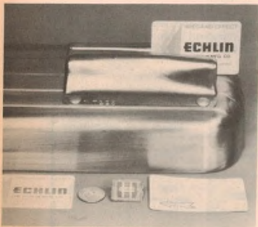
Double row of tiny Wiegand wires embedded in plastic card (foreground) produces pulses when passing magnets in a reader. Wire codes can't be altered.
