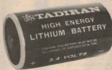
This Tadiran "D" size lithium cell is typical of the present state of the art. Generating 3.4V on load it has a capacity of 10Ah at 60mA.
