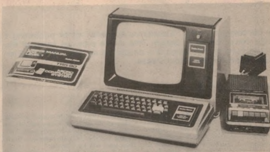
Here is the prize: a TRS-80 Level 1 personal computer system complete with power supply, 30cm video monitor, cassette tape recorder and the widely-acclaimed Level 1 User's Manual.
