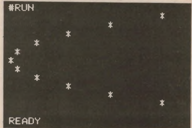
Fig. 1: By using the PRINT TAB command, you can get your computer to plot a simple graph, like this parabola.
