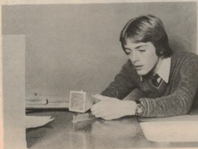
Brad Garnham aims the receiving antenna to receive microwave energy reflected from an aluminium screen.
