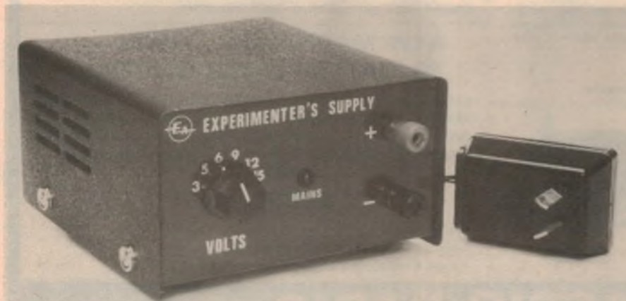
Here is the completed prototype together with the 12V AC plugpack. The unit is totally isolated from the mains in the interests of safety.
