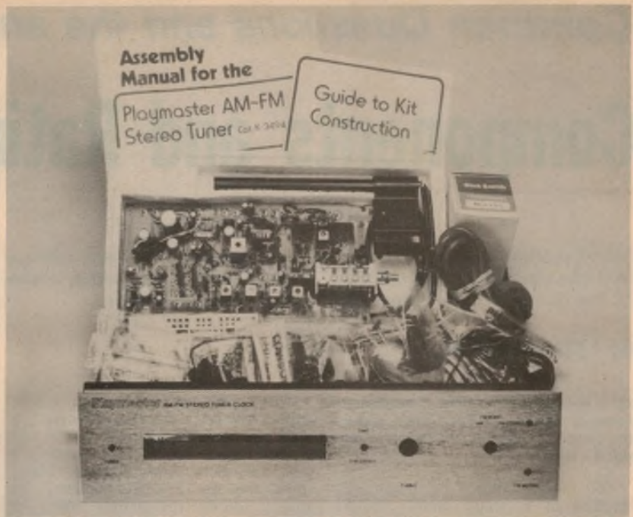
This AM-FM stereo tuner kit from Dick Smith Electronics comes complete with a pre-punched steel chassis and an anodised scratch-grain-finished front panel.
