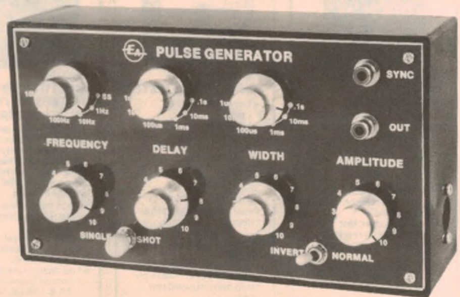
The finished instrument is housed in a neat plastic box and the "Scotchcal" label gives it a professional appearance. Note that the switches and pots for each function are grouped together for ease of operation. The socket in the right hand end is the 12V AC inlet from the plug-pack.
