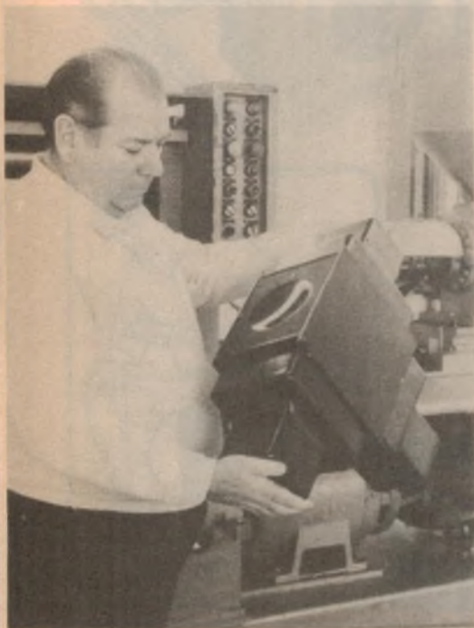
AQUABEAM SYSTEM uses dichroic mirrors to combine colour images from three tubes into a single beam, which is projected through a single lens onto the screen. Art Tucker (at left) is shown holding the housing for the 3-tube assembly.
