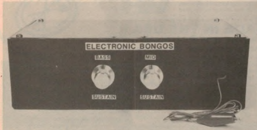
Two potentiometers allow the Bongos to be individually tuned.
