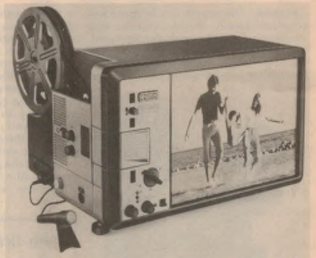
The Eumig S912GL sound projector, which offers a 12V/100W lamp, 180m spool capacity and "optical levelling": the front lens element is moved to centre the picture on the screen.
