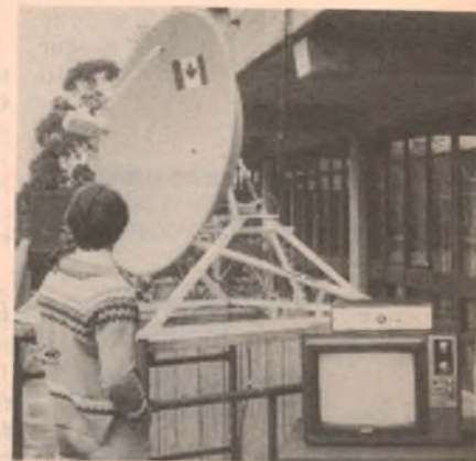
Above: pointing directly at the Hermes satellite, this small earth terminal was used to receive live TV signals during a recent Canadian demonstration.
