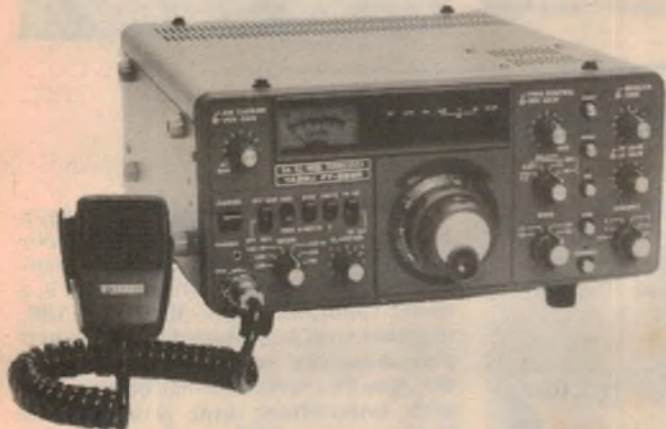
The Yaesu F625RD. The dial is fitted with a skirt, behind the larger knob, which reads units and 10s of kHz, and a window, just above the skirt, which reads 100s of kHz
