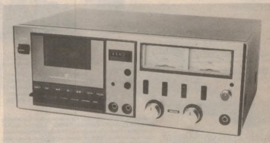
Teac's auto-bias feature consists of a motor driven potentiometer which varies the bias while the response to a 10kHz signal is measured.
