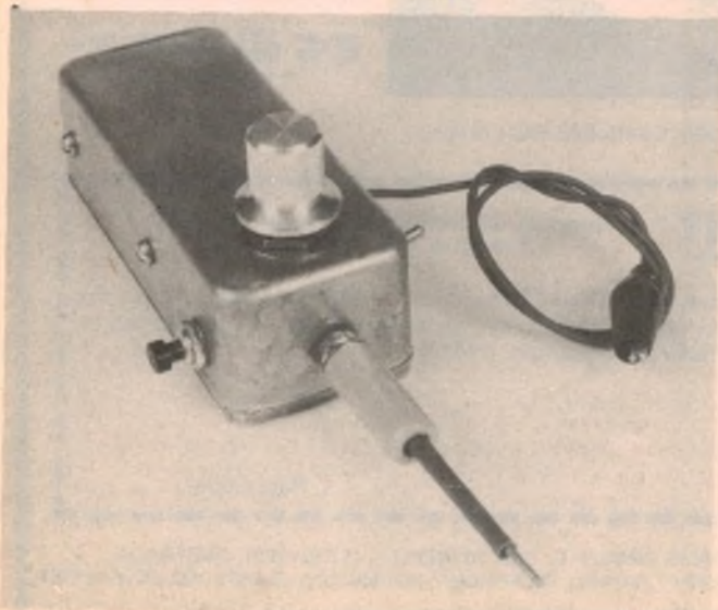
A diecast metal case was used to house the prototype. The probe was made from a stout piece of tinned-copper wire soldered to the centre lug of a jack plug.
