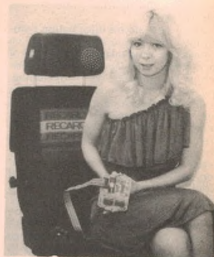
Computer-controlled seat adjustment system from Recaro and National Semiconductor. The seat automatically adjusts to one of two pre-programmed positions at the press of a button.
