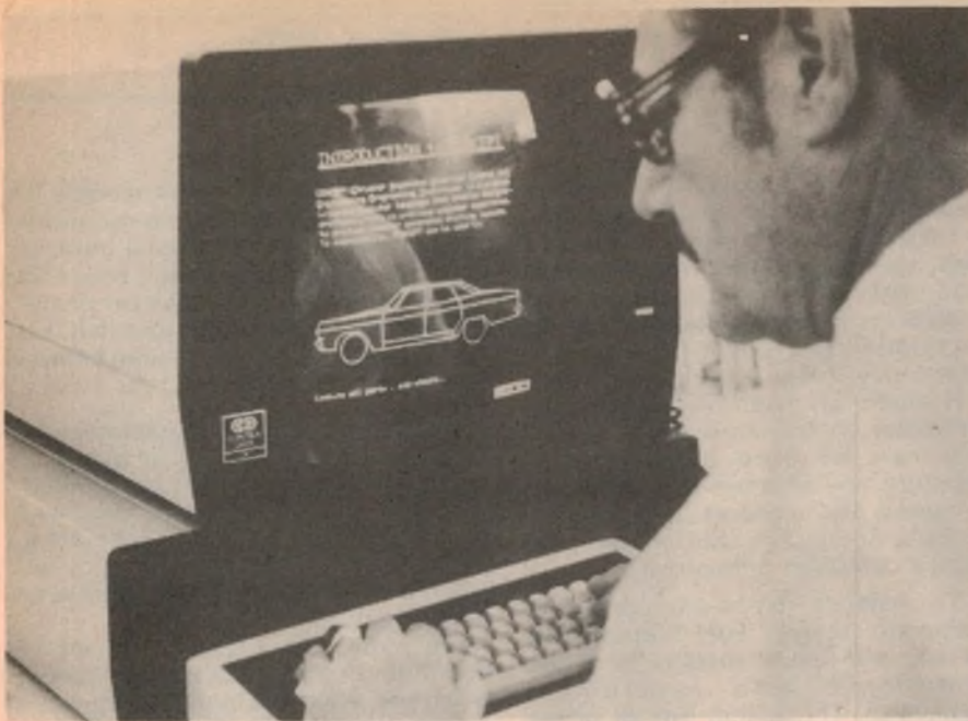
A Chrysler engineer uses a colour graphics terminal to analyse a car body design. Computers will help Chrysler meet stringent new government regulations.
