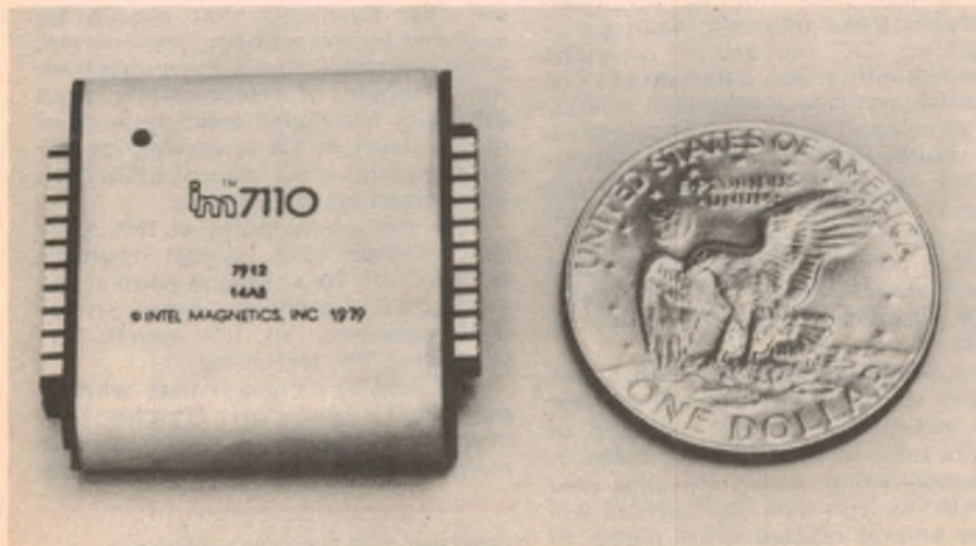
Intel Magnetics 7110 1-megabit magnetic bubble memory device.
