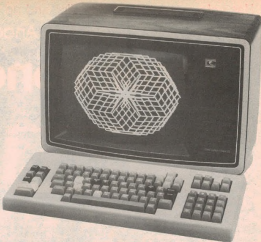
Shown above is the Compucolor II with an extended keyboard. The "spirograph" pattern on the screen shows the graphics capability of the Compucolor.
