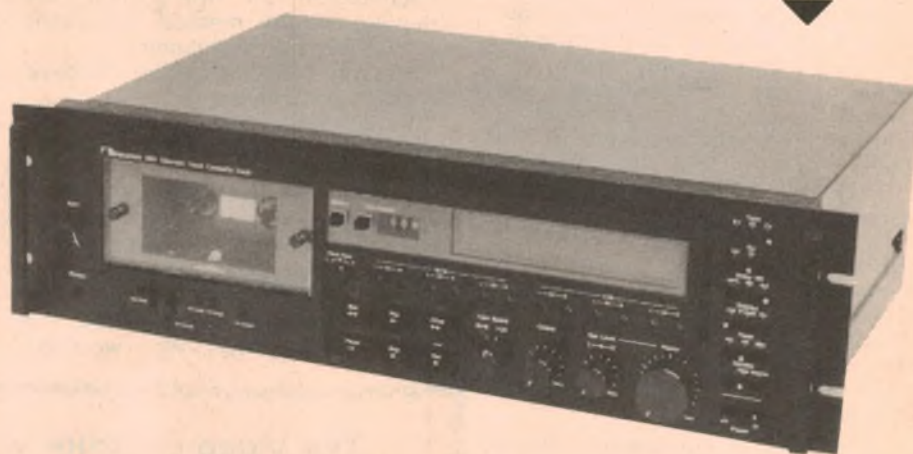
The new Nakamichi 680 cassette deck. The front panel is finished in matte black with white lettering. The rack mounting brackets can be readily removed, if not required.
