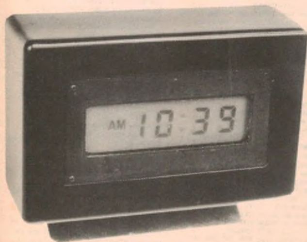
The desk clock version (above) was powered from a 1.5V penlite cell. The circuit diagram at right also shows how the unit and the display light can be powered from a car battery.
