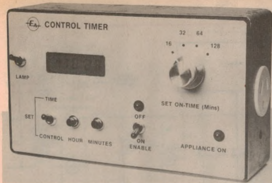
The Control Timer can be set to switch on a mains-powered appliance at a pre-determined time for a period of 16, 32, 64 or 128 minutes.
