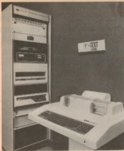
Above: the teletext equipment rack and control console. Included in the rack are a teletext data encoder/decoder, a DEC RK105 cartridge disc system, a DEC twin-deck floppy disc system, and a PDP 11/34 minicomputer.
